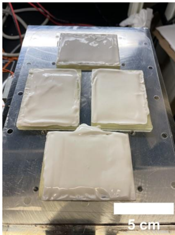
Figure S2. Freeze casting of YSZ slurry into molds on the surface of the thermoelectric cold plate.
