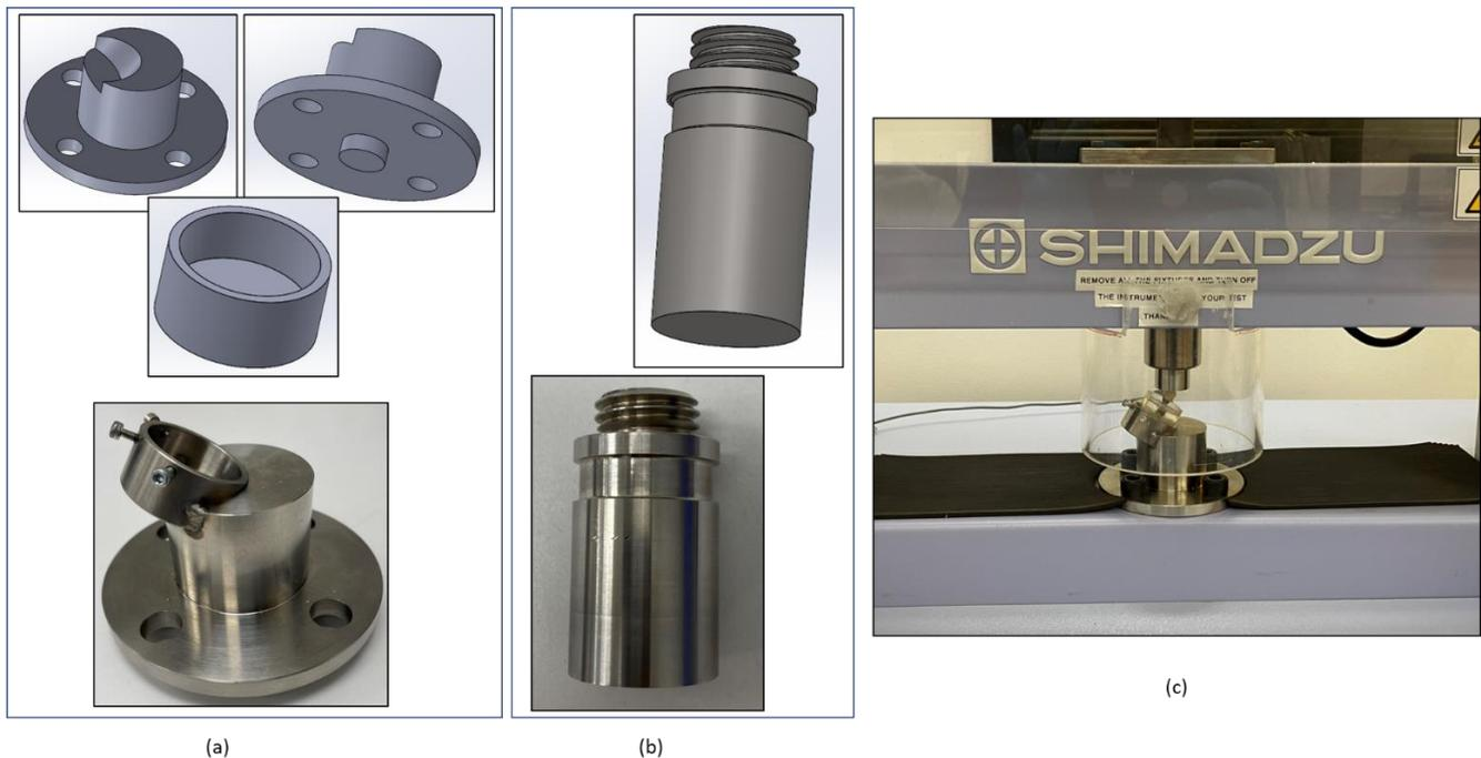
**Figure 7.** (a) Custom Shimadzu 30-degree fixture (top: CAD model; bottom: milled part). (b) Custom flat metal piston (top: CAD model; bottom: milled part). (c) Oblique load test setup.
