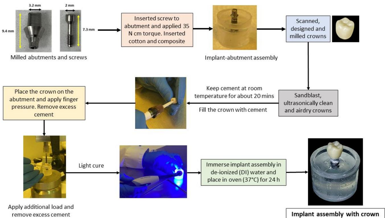
**Figure 4.** Abutment placement and cementation procedure on the implant assembly.
