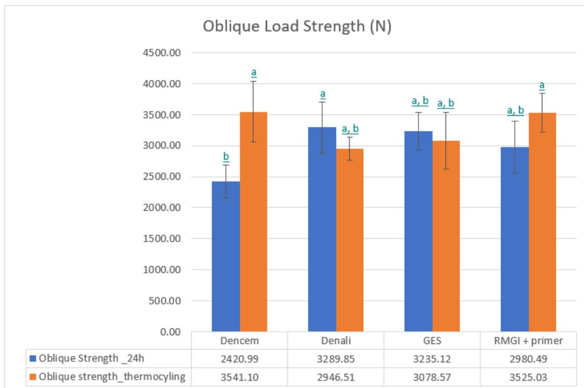
**Figure 10.** Oblique load test data of the implants with different cements (blue) after 24 h of the samples placed in DI water at 37 °C and (orange) after thermocycling the samples for 9 days ( $p < 0.05$ ). The bars that do not share a letter have a significant difference among their respective means, as per the Tukey pairwise comparison test (95% confidence).
