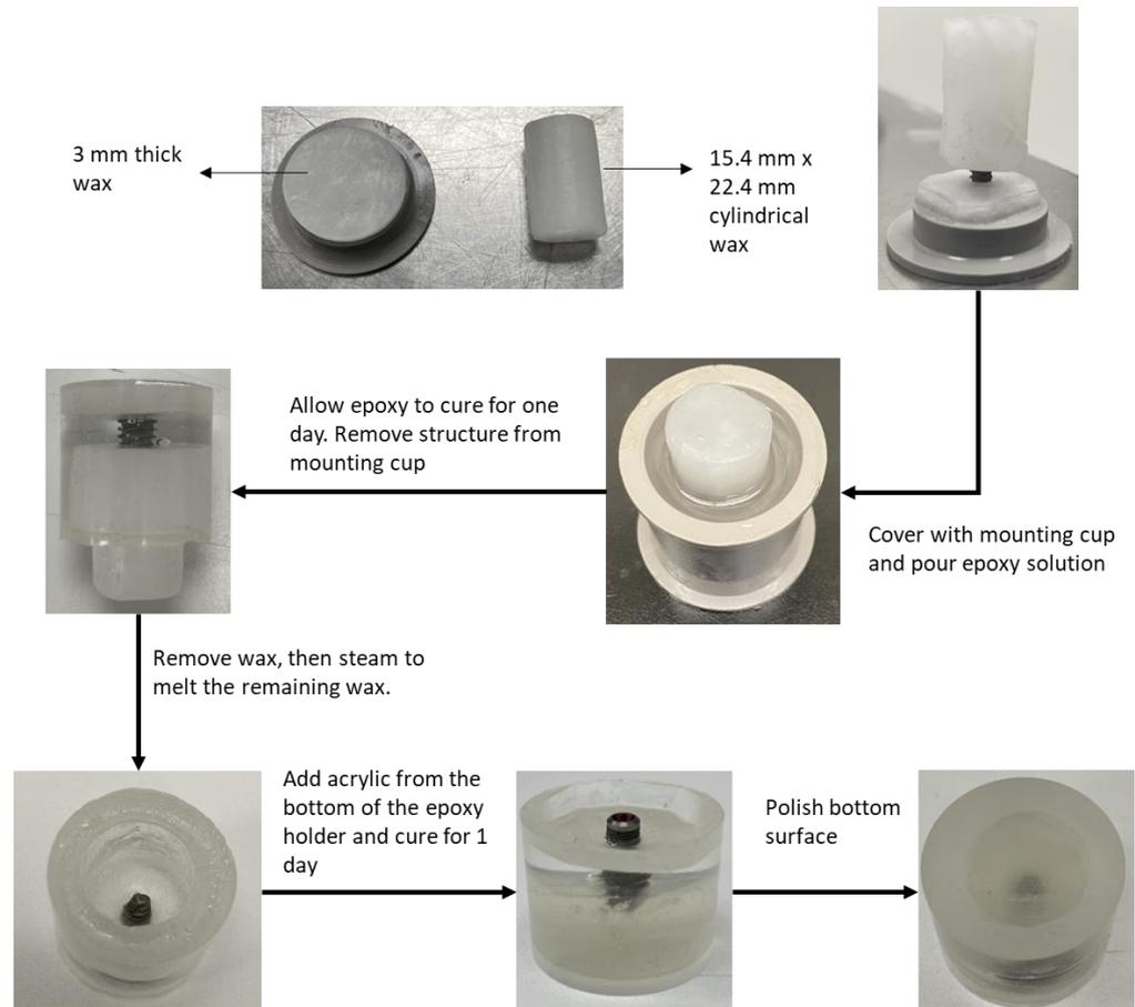
**Figure 3.** Step-by-step procedure for preparing the bi-layered holder and embedding the implant body in the holder.
