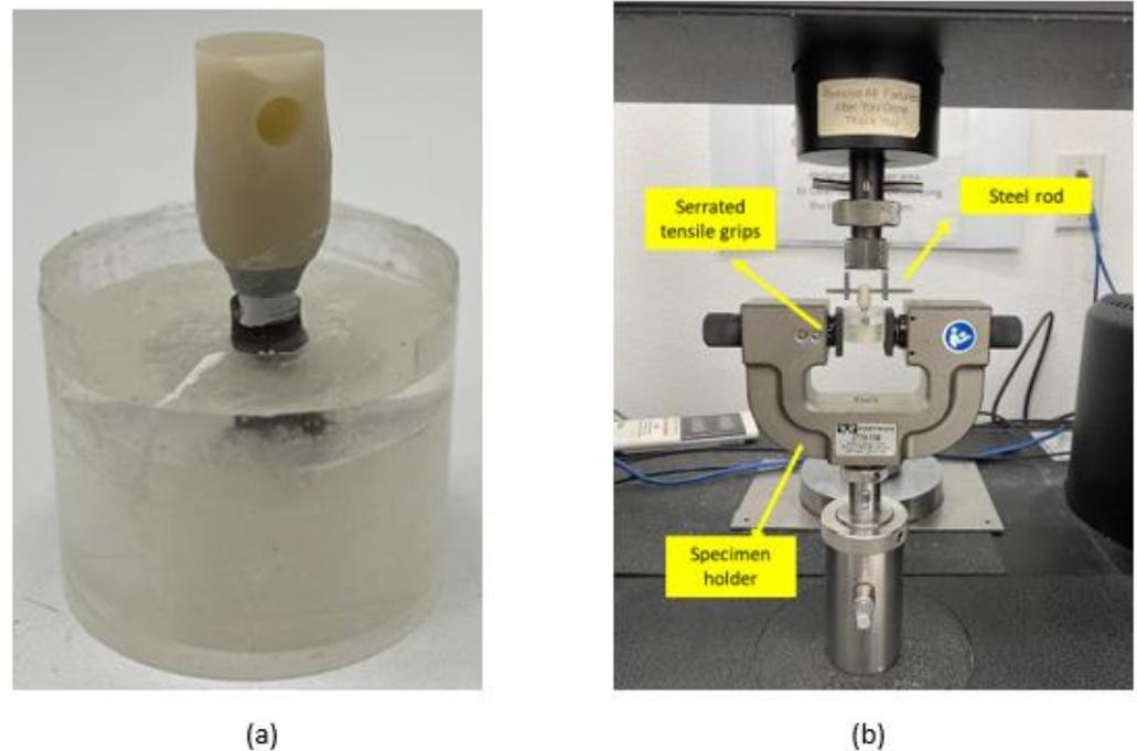
**Figure 5.** (a) Implant assembly used for tensile bond strength tests of the cements. (b) Tensile bond strength test setup.
