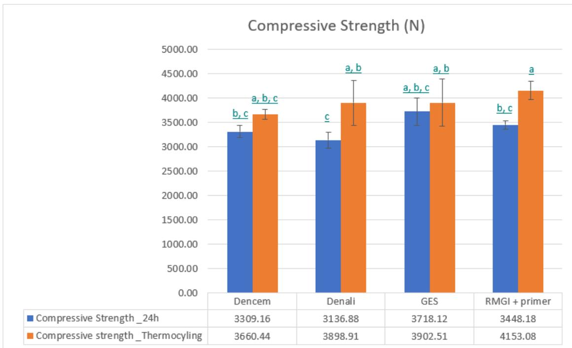
**Figure 9.** Compressive load test data of the implants with different cements (blue) after 24 h of the samples placed in DI water at 37 °C and (orange) after thermocycling the samples for 9 days ( $p < 0.05$ ). The bars that do not share a letter have a significant difference among their respective means, as per the Tukey pairwise comparison test (95% confidence).
