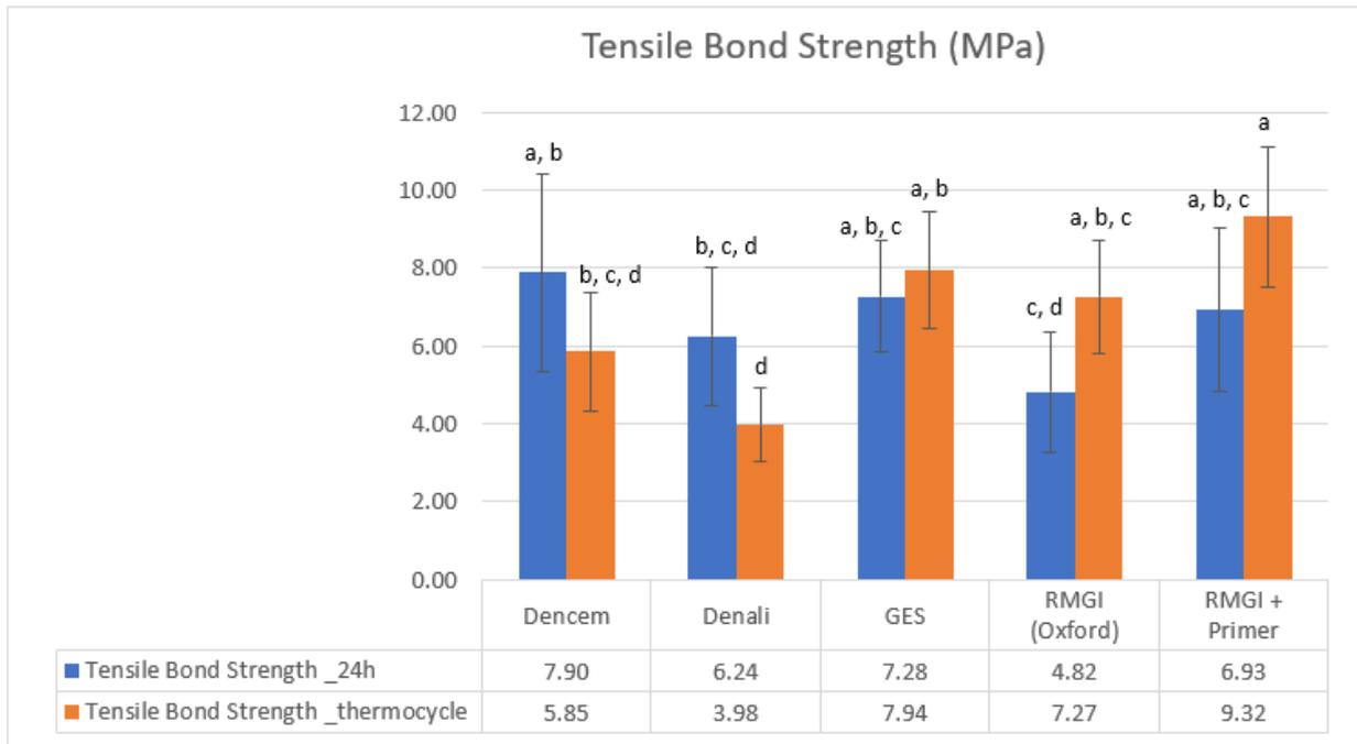
**Figure 8.** Tensile bond strength of the cements (blue) after 24 h of the samples placed in DI water at 37 °C and (orange) after thermocycling the samples for 9 days ( $p < 0.05$ ). The bars that do not share a letter have a significant difference among their respective means, as per the Tukey pairwise comparison test (95% confidence).
