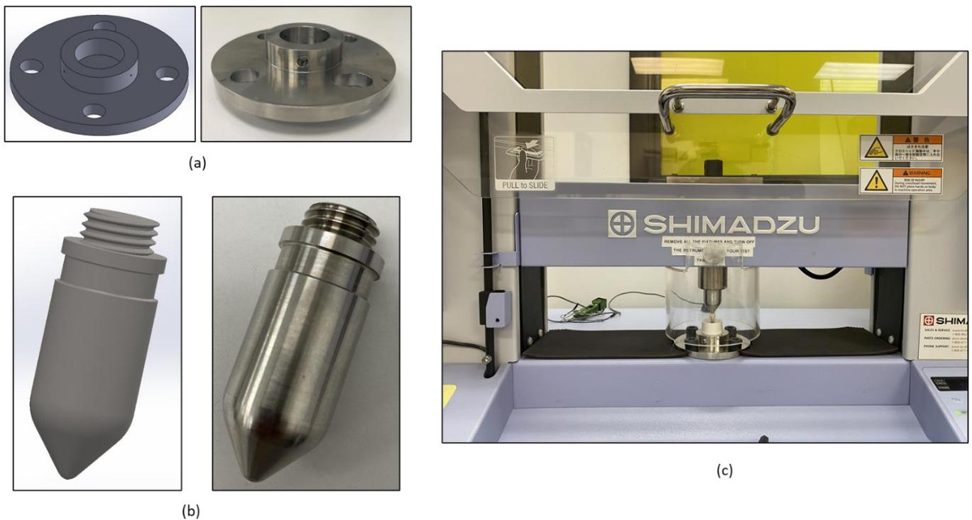
**Figure 6.** (a) Custom Shimadzu fixture (left: CAD model; right: milled part). (b) Custom metal piston (left: CAD model; right: milled part). (c) Compressive load test setup.
