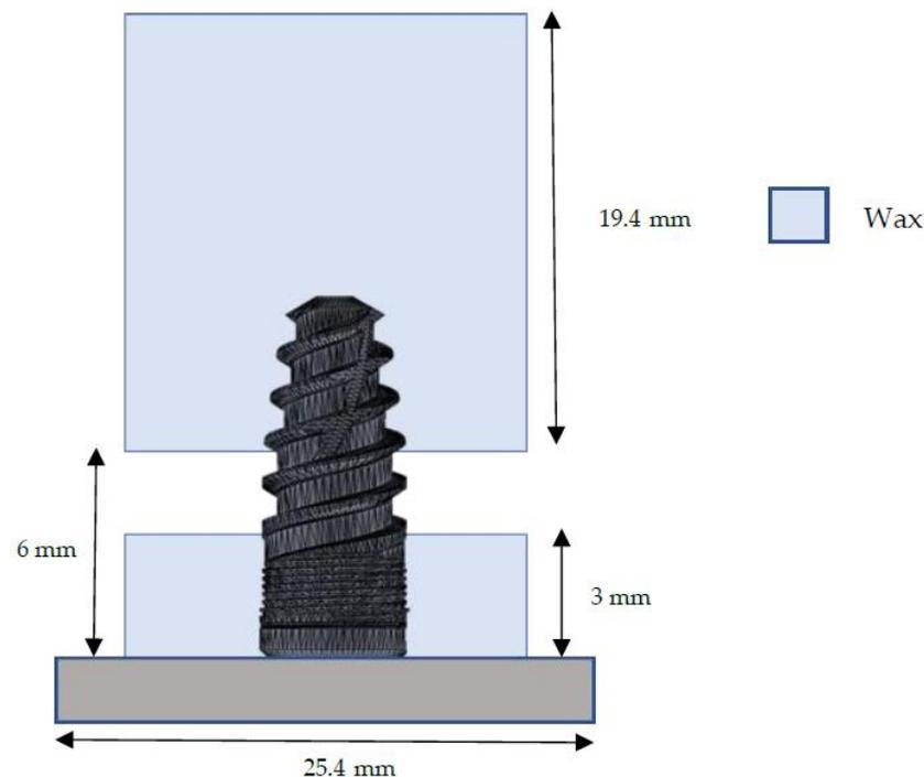
**Figure 2.** Schematic of the implant body placement in the mounting cup. The regions left out were covered by epoxy. After the epoxy was cured, the wax was removed and replaced with acrylic.
