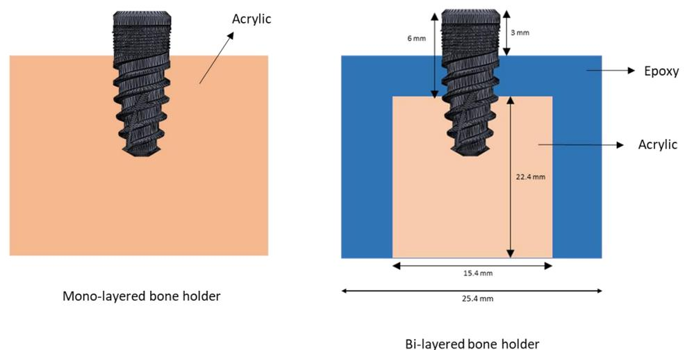
**Figure 1.** Mono- and bi-layered artificial bone holders.
