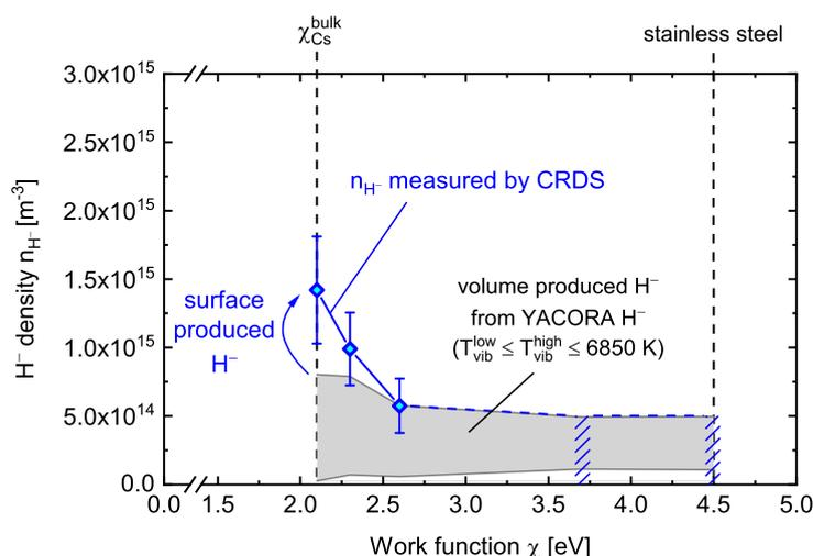
**Figure 4.** The negative hydrogen ion density measured by cavity ring-down spectroscopy system (CRDS) is shown for different work functions. The gray shaded area shows possible values for the density of negative ions created by volume processes and obtained from YACORA  $\text{H}^-$ .
