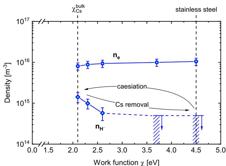
**Figure 3.** Negative hydrogen ion and electron densities measured for different work functions in a hydrogen plasma at 2 Pa and 450 W. The measurements are taken at 2 cm and 8 mm from the sample surface, respectively.
