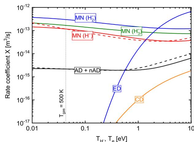
**Figure 1.** Rate coefficients of the different  $H^-$  destruction processes, calculated from the cross sections in [29] as functions of the electron temperature for the electron detachment process and of the  $H^-$  temperature for the other processes. Solid lines correspond to fixed temperatures for neutral particles and positive ions of 500 K, while the dashed lines correspond to  $T_H = T_{H^+} = T_{H^-}$ .
