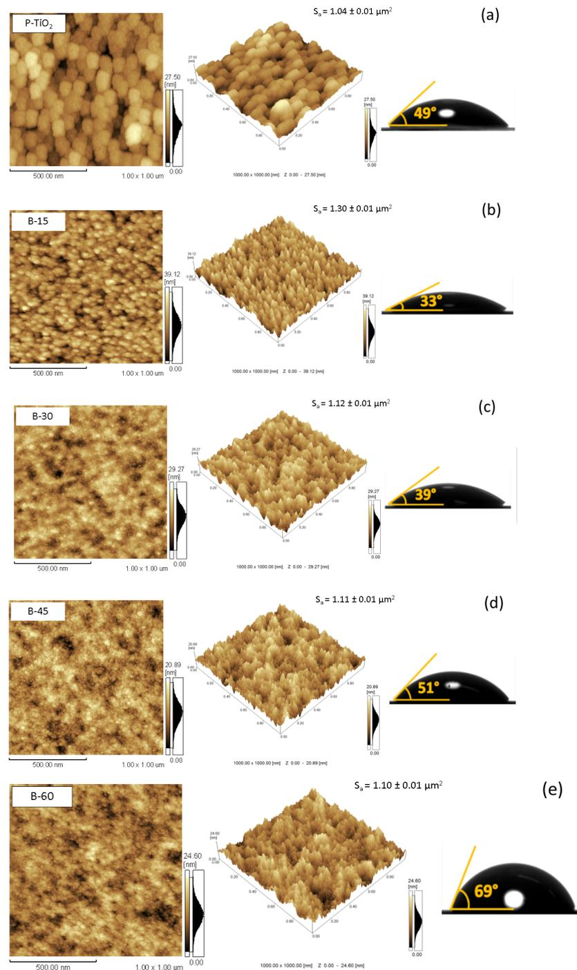
**Figure 1.** AFM 2D and 3D images, alongside water droplet photographs depicting the contact angles formed with the surface of (a) pristine and black TiO<sub>2</sub> films treated in the HCHP process for durations of (b) 15, (c) 30, (d) 45, and (e) 60 min. For each sample, the surface area (S<sub>a</sub>) obtained by AFM measurements is presented.
