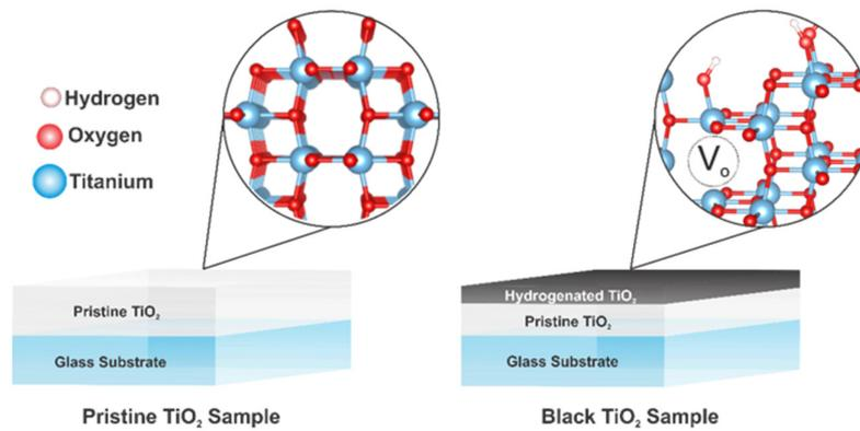
**Figure 3.** Schematic illustration of the pristine and black  $TiO_2$  thin films, emphasizing their microstructures and the hydrogenated layer following HCHP treatment.
