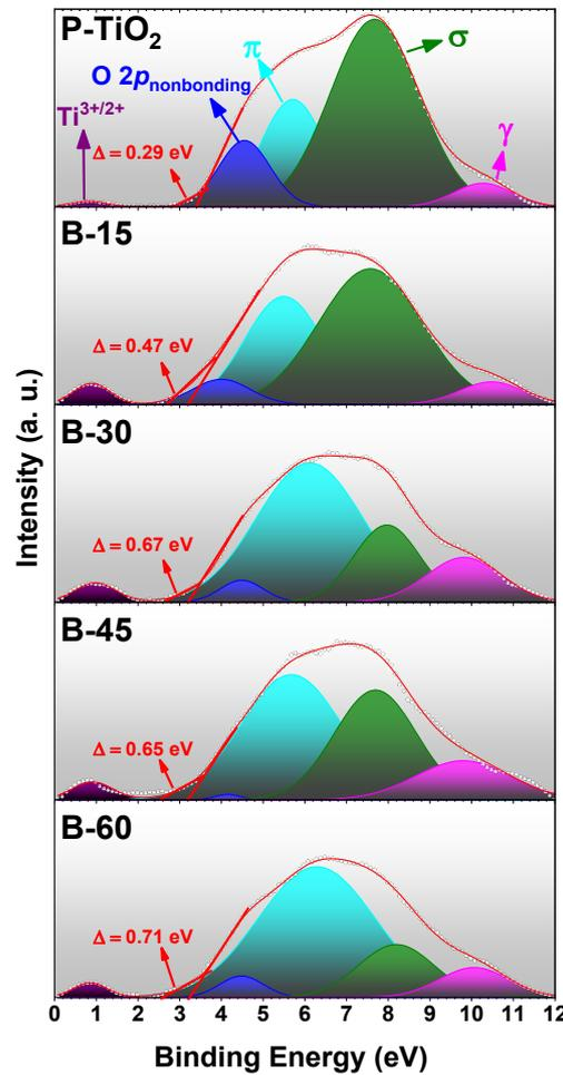
Figure 7. XPS valence band spectra were obtained for both pristine and black  $TiO_2$  thin films subjected to the HCHP process for durations of 15, 30, 45, and 60 min.
