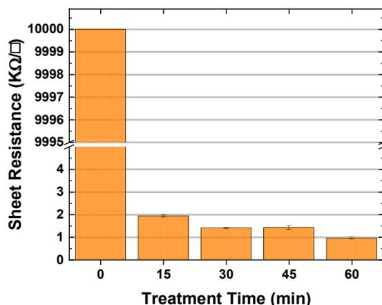
Figure 9. Sheet resistance (in  $\text{k}\Omega/\square$ ) values as the HCHP treatment time increases.
