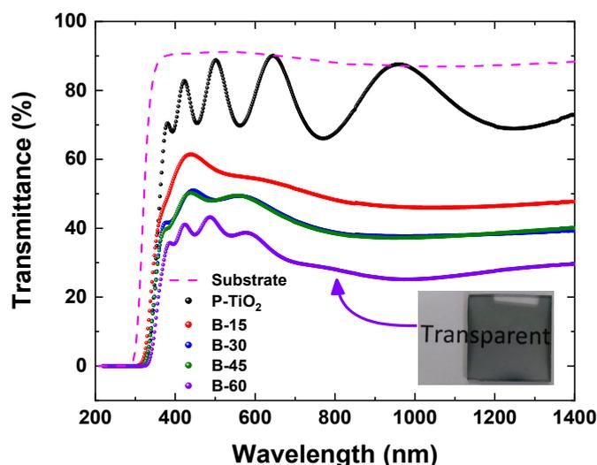
**Figure 6.** The UV-Vis-NIR transmittance spectra were obtained for glass substrates, both pristine and black  $TiO_2$  thin films, which were hydrogenated using the HCHP process for durations of 15, 30, 45, and 60 min.
