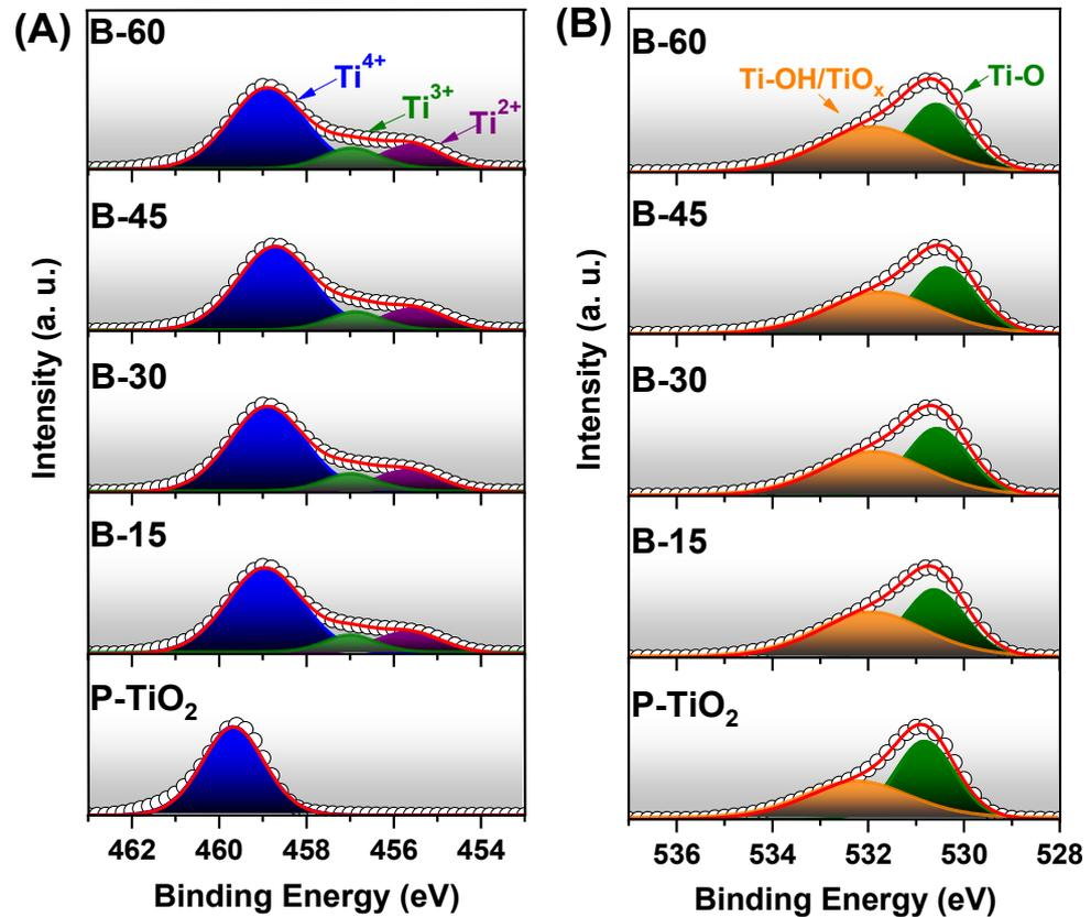
**Figure 5.** High-resolution XPS spectra of (A)  $Ti\ 2p_{3/2}$  and (B)  $O\ 1s$  peaks of each sample before and after the HCHP process during 15, 30, 45, and 60 min. Open circles and lines represent the experimental data and the fit, respectively.
