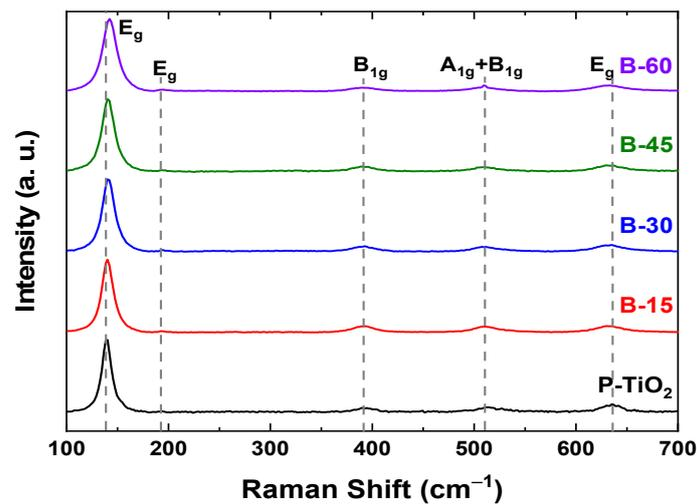
**Figure 4.** Raman spectra of the samples, highlighting the main anatase vibrational modes.
