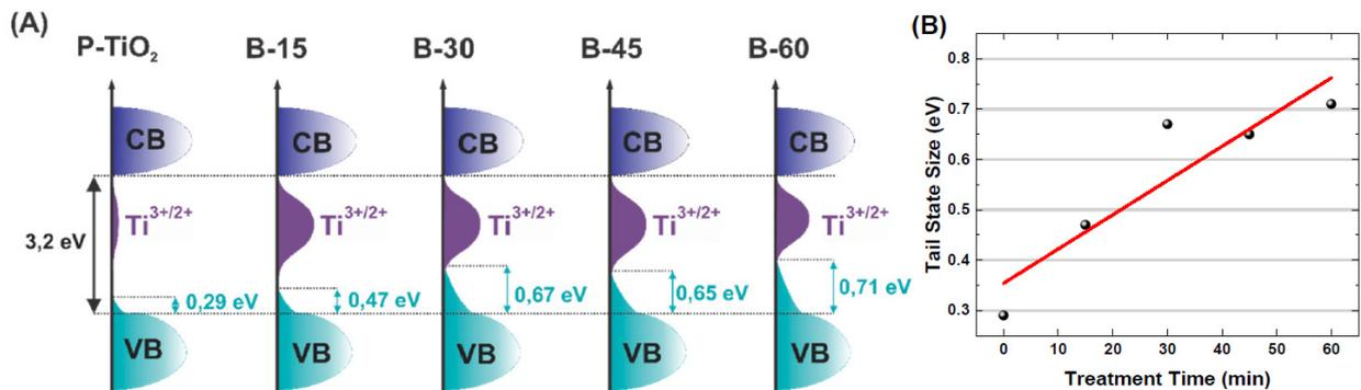
Figure 8. (A) Schematic representation of defect  $Ti^{3+/2+}$  and tail states occurring between the valence and conduction bands; (B) the increase in tail state size as a function of HCHP treatment time, with the red line representing a linear fit.
