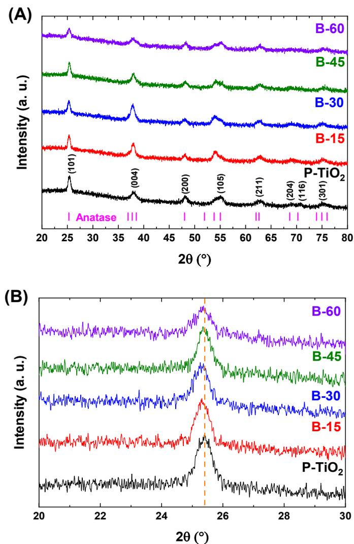
**Figure 2.** (A)  $TiO_2$  anatase XRD patterns. (B) Magnified XRD patterns of (101) plane for pristine  $TiO_2$  and B- $TiO_2$  thin films treated for different durations.
