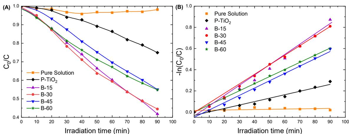
**Figure 10.** (A) MB photodegradation comparison over pristine  $TiO_2$  and black  $TiO_2$  hydrogenated by different conditions under UV light; (B) determination of rate of constant via  $-\ln(C_0/C)$  vs. time plot for photocatalytic degradation of MB system under UV light.
