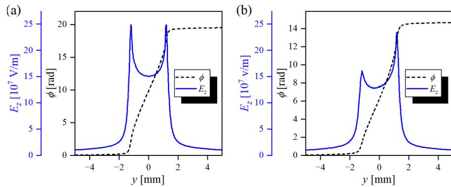
**Figure 12.** Numerical simulations of the  $z$ -component of the electric field (full blue line) with the calculated rise in the phase shift (dashed black line) due to the Kerr effect along the path (of the laser beam) perfectly aligned with the  $y$ -axis (a), and along the path that slightly leaned in the  $z$ -direction causing apparent field distortion (b). The electrode voltage in the simulation is 160 kV.
