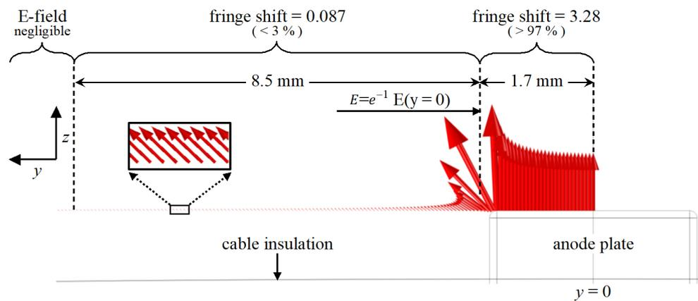
**Figure 5.** Estimation of contribution to the total phase shift of the probing beam at a voltage of 150 kV in the areas where the electric field is appreciable. Distribution of electric field around the anode plate in the  $y$ - $z$  plane is indicated by the red arrows.
