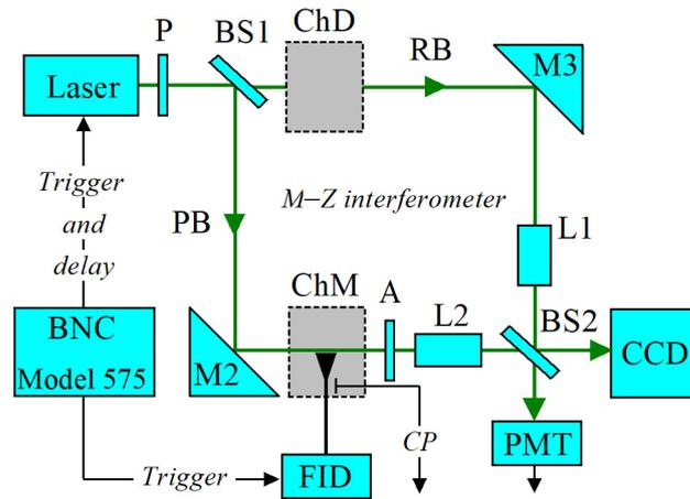
**Figure 2.** Block scheme of the interferometric (Mach-Zehnder) setup: P—polarizer; A—analyzer; M1 and M2—mirrors; RB—reference beam; PB—probing beam; ChD—delay chamber; ChM—measurements chamber with the plate anode; BS1 and BS2—beam splitters; PMT—photomultiplier; L1 and L2—objective lenses; FID—high-voltage pulsed source; CP—signal from the capacitive probe.
