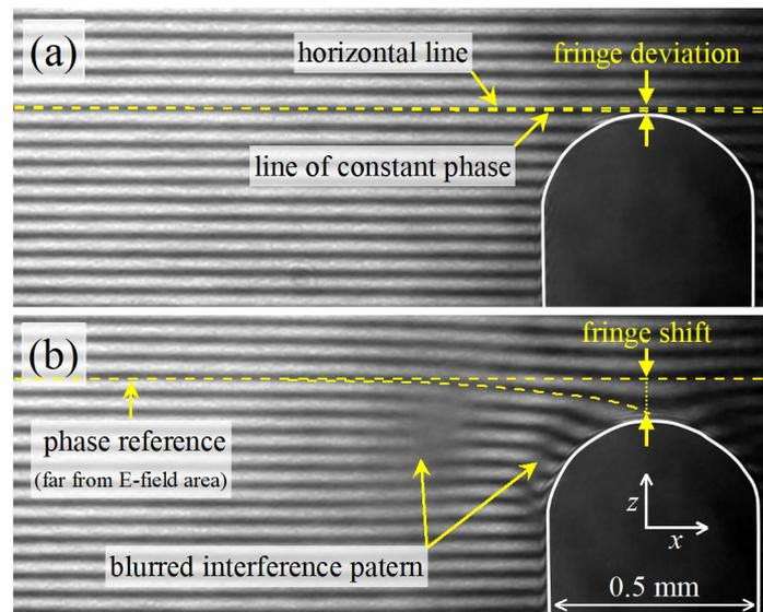
**Figure 7.** Description of fringe pattern in a typical interferogram: fringe deviation at zero field due to optical system distortion (a) and fringe pattern destruction and shift due to electric field (time delay from the voltage pulse onset and voltage are 3 ns/154 kV) (b). The anode plate edge is outlined for better visibility. Vertical laser polarization.
