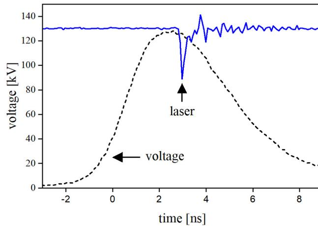
**Figure 3.** Typical waveforms of voltage acquired by the capacitive probe and the photomultiplier detecting the laser pulse.
