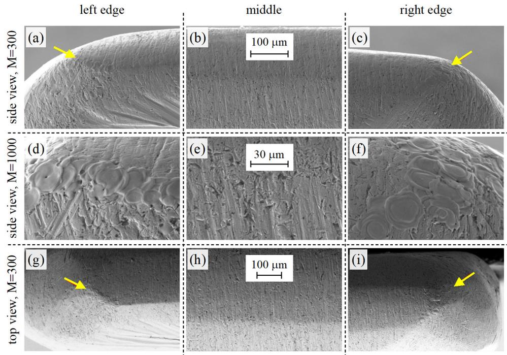
**Figure 9.** Morphology of the electrode tip in the central area and edges. Macroscopic views (a–c,g–i) and detail (d–f). Yellow arrows in (a,c,g,i) point to the path on which the discharge was evidently preferentially formed.
