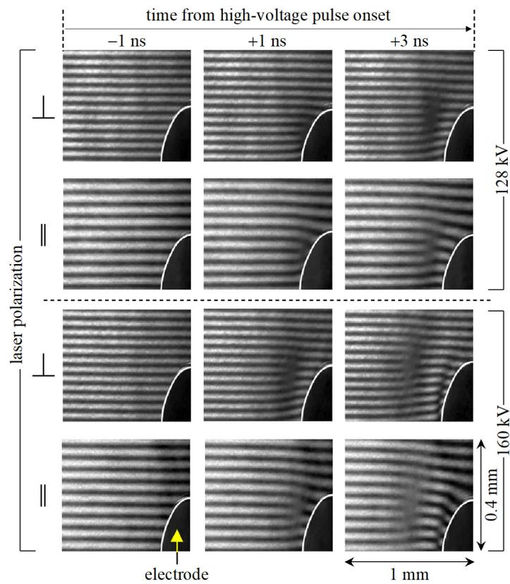
**Figure 10.** Series of interferograms demonstrating fringe distortion at different voltages and laser polarizations. The images do not preserve the original aspect ratio (larger horizontal scale) for better fringe shift visibility. The interferometer is set up such that the fringes always shift in the presence of electric field towards the electrode at the axis of symmetry.
