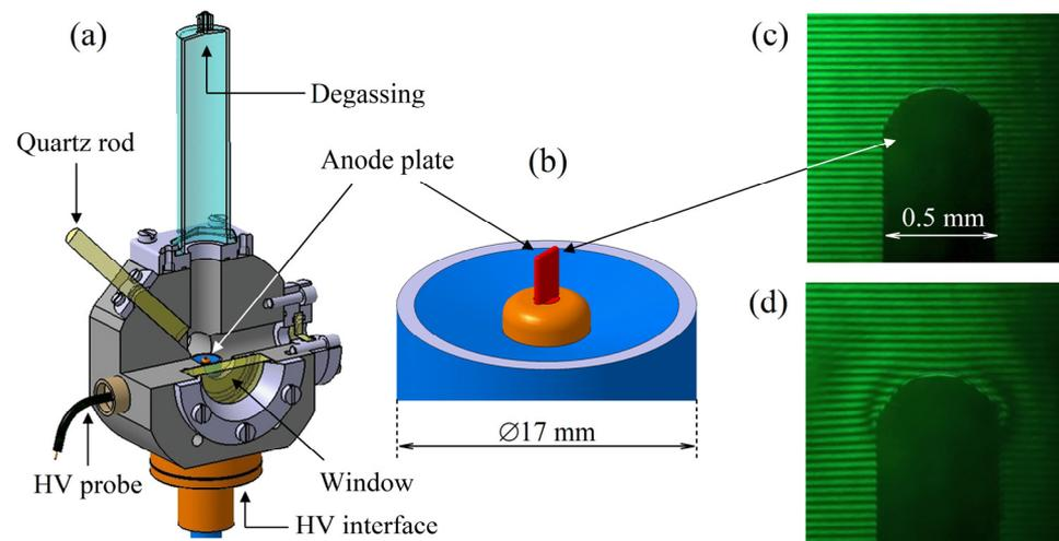
**Figure 1.** Simplified sketch of (a) the reactor chamber composed of a grounded stainless-steel body, windows for optical diagnostics, and a water inlet/outlet, and (b) the coax-based HV electrode (plate anode). Images (c,d) show examples of interferograms near the plate anode (visible as the dark silhouette) captured at zero voltage (c) and at 160 kV (d).
