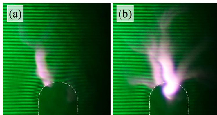
**Figure 8.** Examples of (a) single-corner discharge and (b) two-corner discharge. Peak electrode voltage is  $\sim 175$  kV and time delay from the voltage pulse onset and laser is approximately 3 ns.
