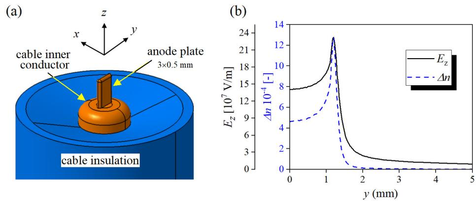
**Figure 4.** Orientation of axes with respect to the plate anode (a) and  $z$ -component of electric field in the  $y$ - $z$  plane calculated at a voltage of 150 kV and corresponding  $\Delta n$  determined by Equation (1) (b). The position of the electrode apex corresponds to  $z = 0$ , and vertical axes of symmetry correspond to  $x = 0$  and  $y = 0$ .
