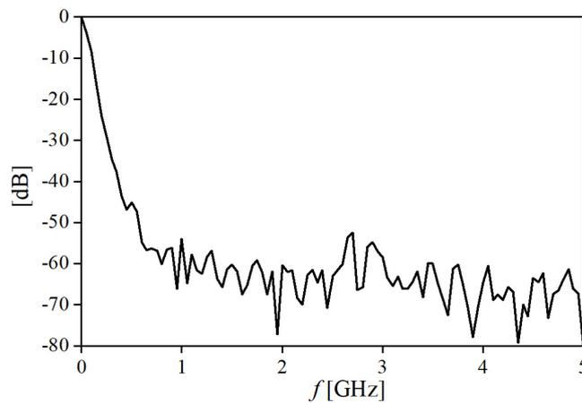
**Figure 6.** Spectrum of the voltage pulse generated by the FID.
