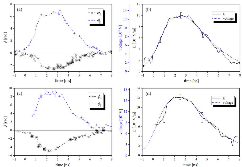
**Figure 11.** Time dependence of phase shift in both laser polarizations (a,c) and corresponding reconstructed electric field waveforms together with the voltage waveforms gained from the HV probe (b,d). The voltage amplitude was 128 kV (a,b) and 160 kV (c,d).
