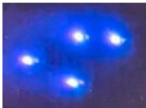
**Figure 10.** Spots expanding on the cathode in the form of a ring with arc current 200 A.
