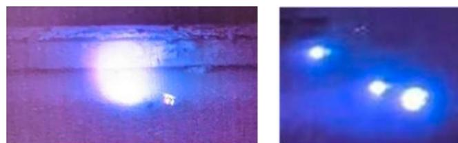
**Figure 1.** Cathode spot view before (left) and after splitting (right) and separation of the new spots away from each other for arc current  $I = 150$  A.
