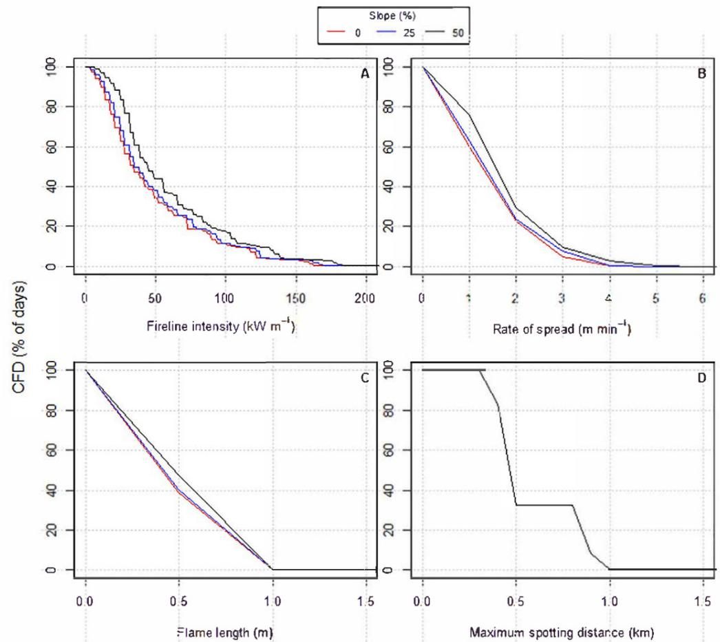
**Figure 6.** Cumulative frequency distribution (CFD) graphs for four fundamental fire behavior characteristics (A–D) based on the Anderson (1982) Fire Behavior Fuel Model 8—Closed timber litter for three different slope steepness levels and 23 years of weather records associated with the fire season at Army Garrison Camp Williams, UT. Upslope fire spread is assumed.
