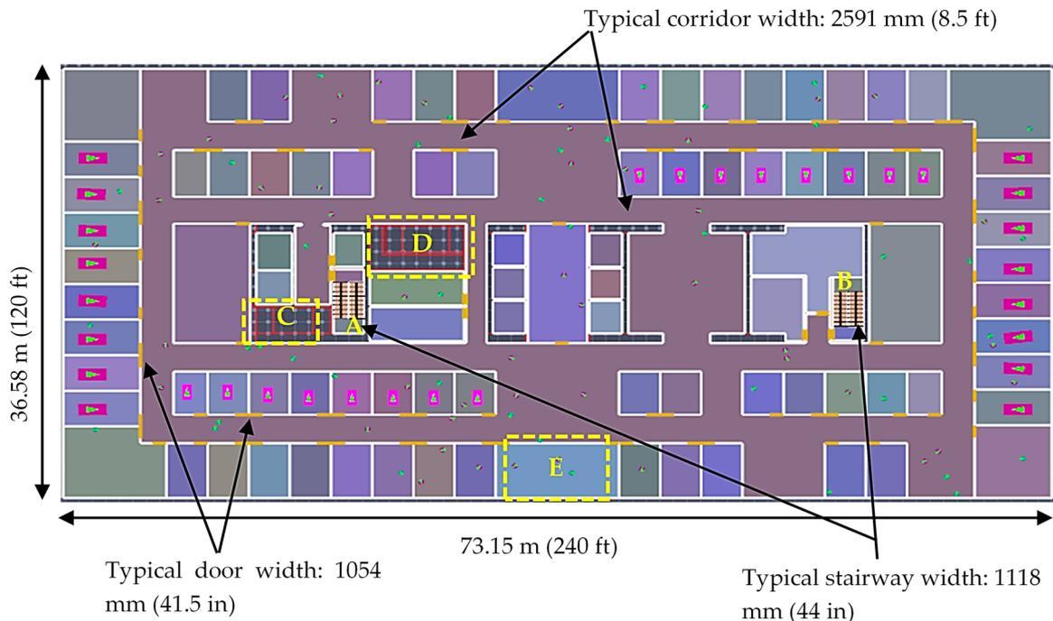
**Figure 3.** Dimensions of egress components as per IBC 2018 [4] and NFPA 101 [5].
