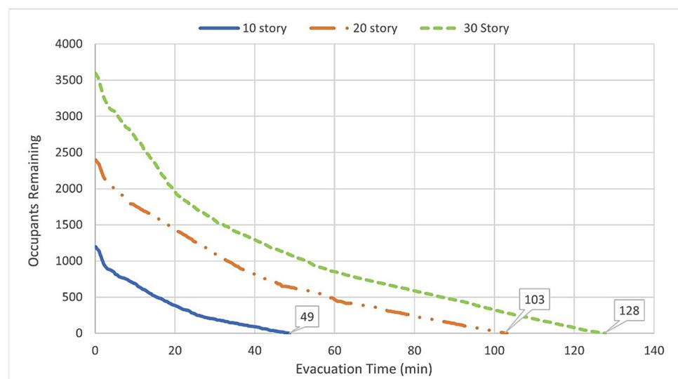
**Figure 4.** Evacuation time with different numbers of stories.
