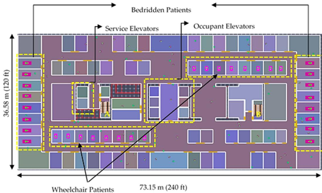
**Figure 1.** Floor plan for the hospital model with two typical stairways required as per IBC 2018 [4] and NFPA 101 [5].
