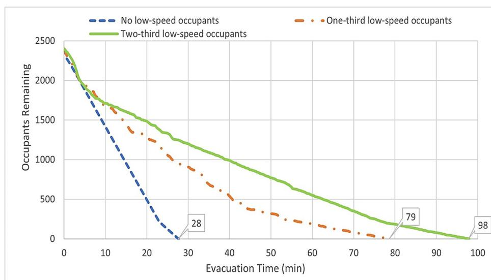
**Figure 8.** Evacuation time with different numbers of slow-moving occupants.
