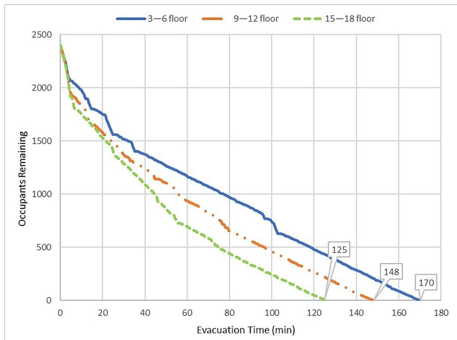
**Figure 9.** Evacuation time with different locations of fire.
