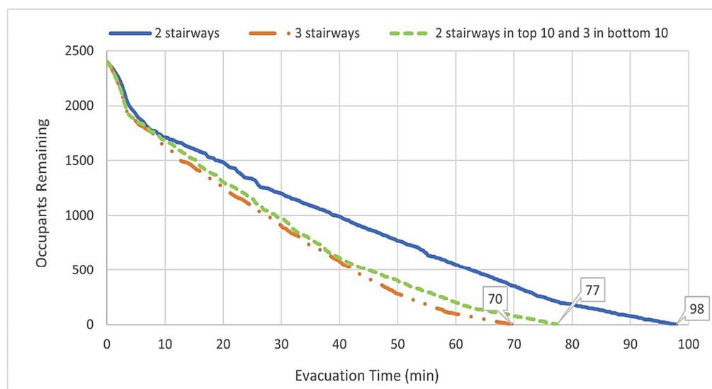
**Figure 6.** Evacuation time with different numbers of stairways.
