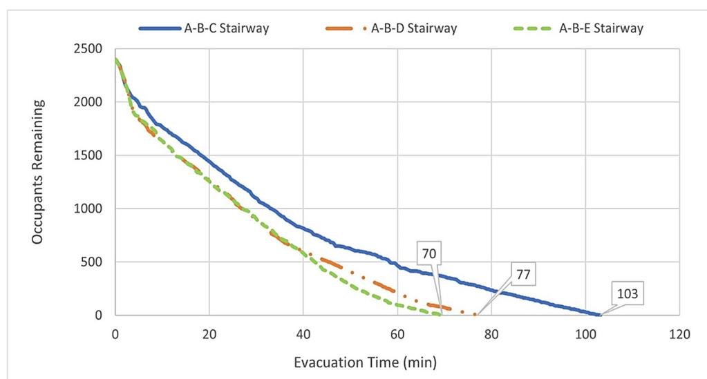
**Figure 5.** Evacuation time with different locations of stairways.
