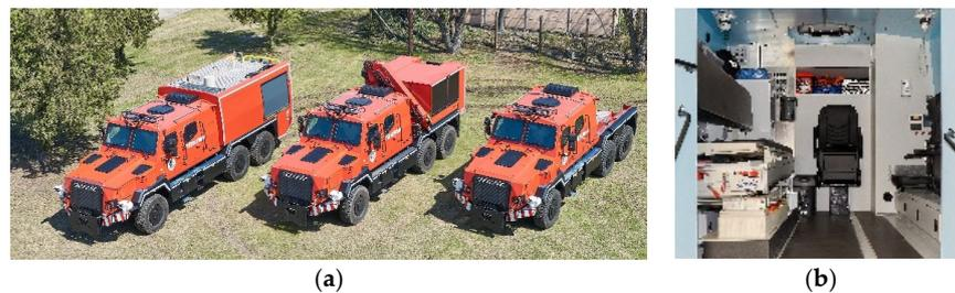
**Figure 3.** RDO 4336 MPV multi-purpose KOMONDOR with a wide range of interchangeable superstructures: (a) exterior image and (b) interior image. Source: author's picture.
