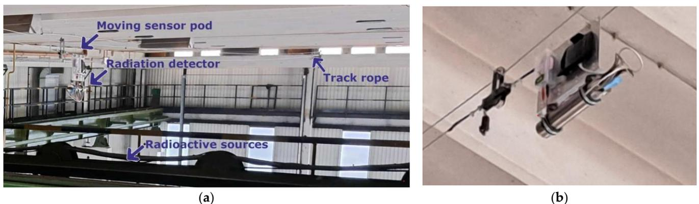
**Figure 9.** (a) Wire ropeway path with a motorised automatic detector moving mechanism. (b) RadNDI scintillation detector attached to the wire ropeway. Source: the author’s own source.
