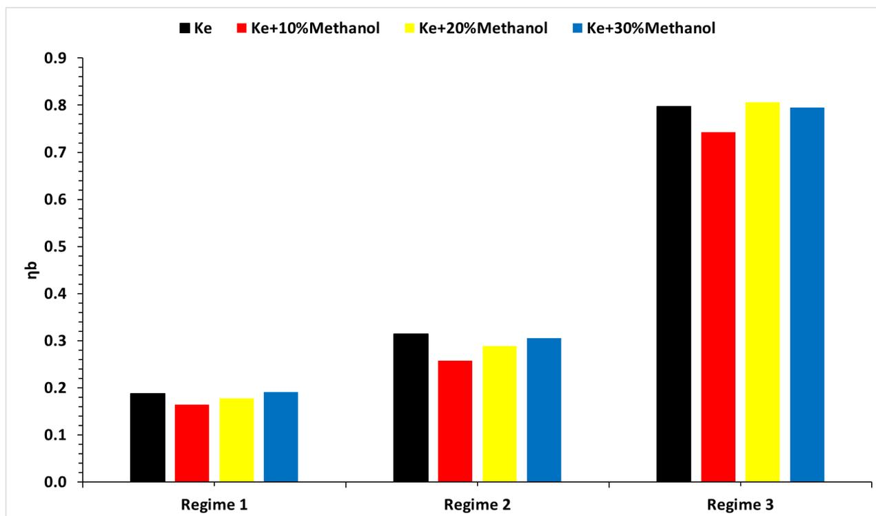
Figure 17. The combustion efficiency vs. regimes and blends.
