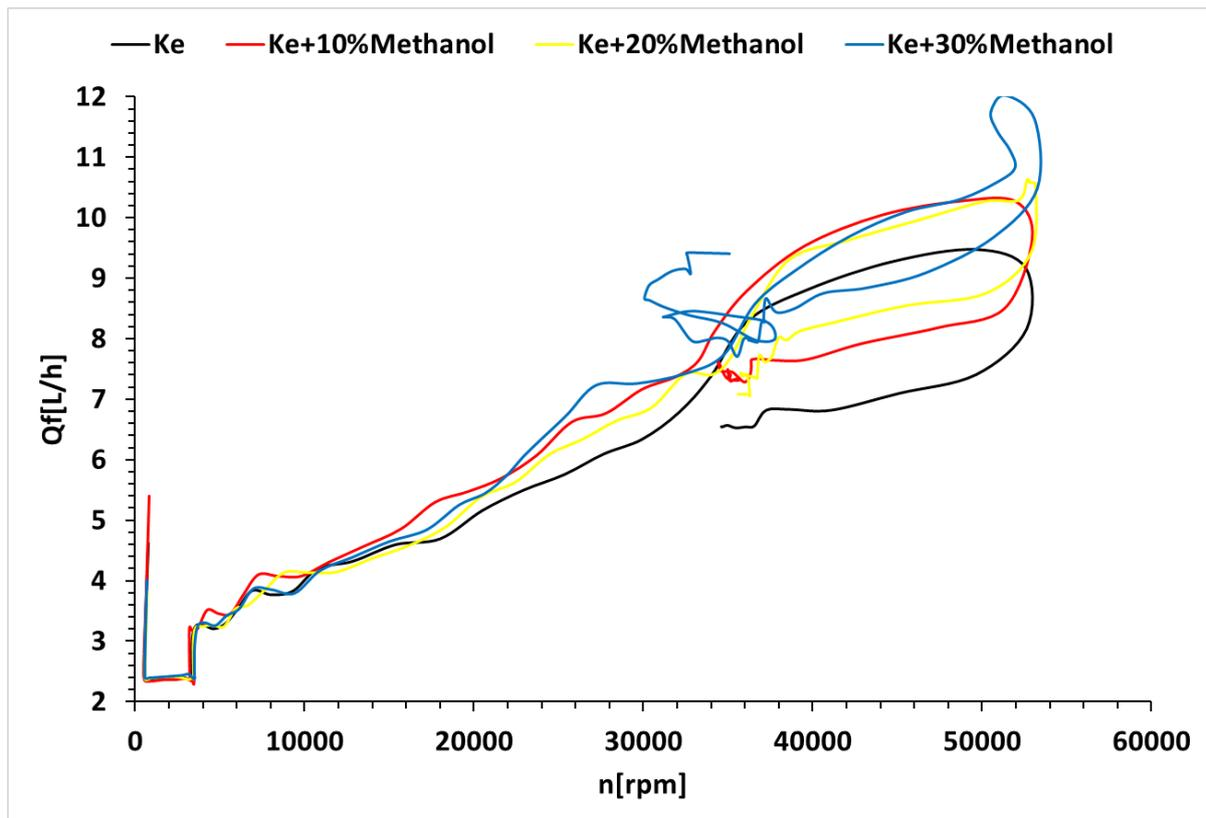
Figure 7.  $Q_c$  (L/h) vs. rpm for different fuel blends during the starting procedure.
