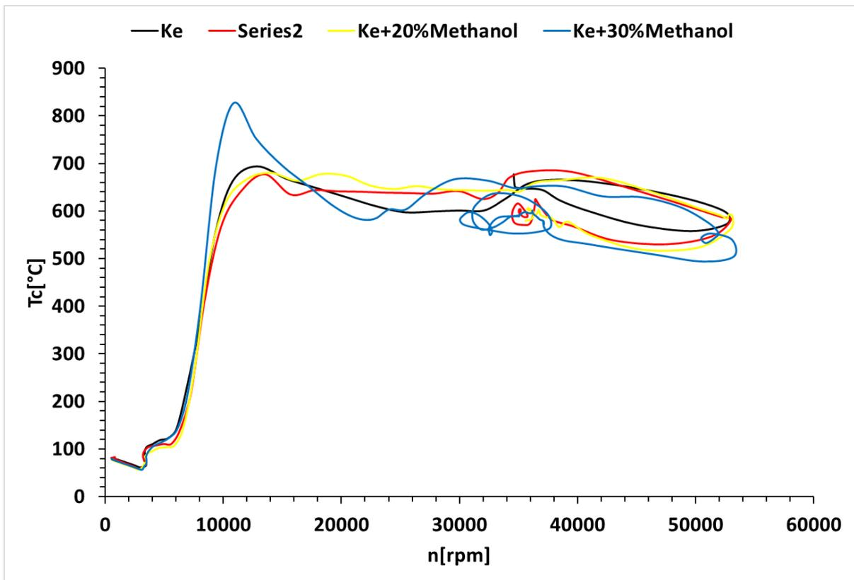
Figure 6. Temperature before the turbine (Tcomb) plotted against rpm for various fuel blends during the starting procedure.
