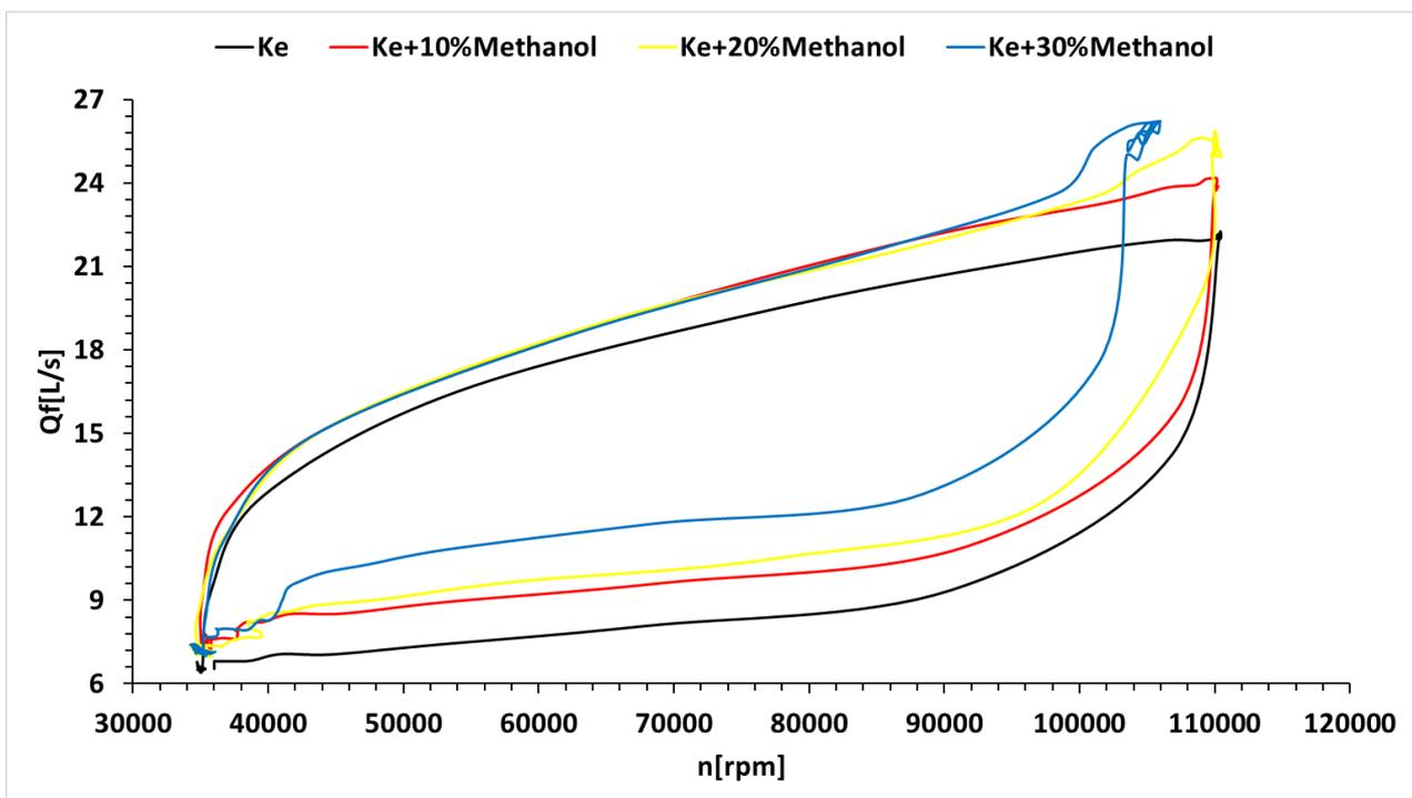
Figure 9. Variation in fuel flow during abrupt acceleration and deceleration.
