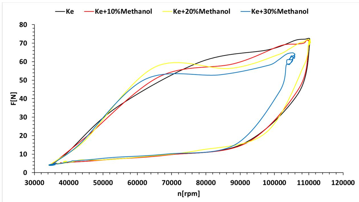
**Figure 10.** Thrust variation during rapid sudden acceleration and deceleration.
