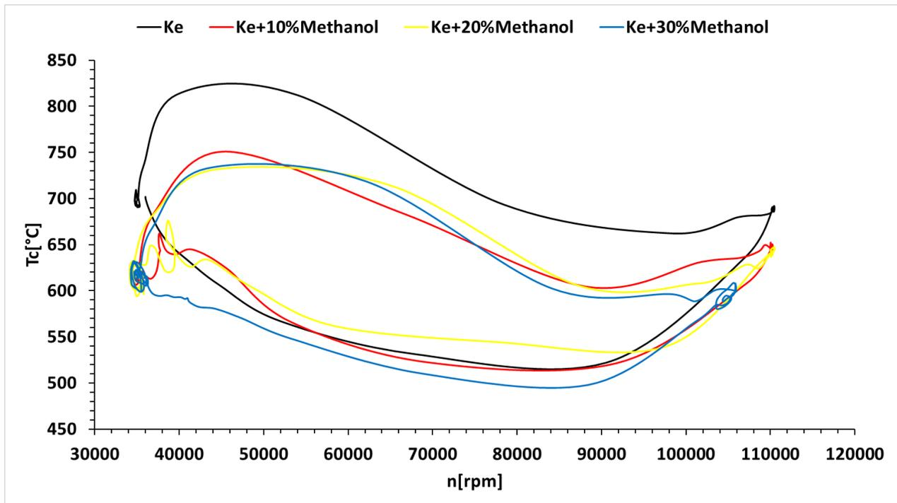
Figure 8. Temperature before the turbine ( $T_{comb}$ ) during rapid acceleration and deceleration.
