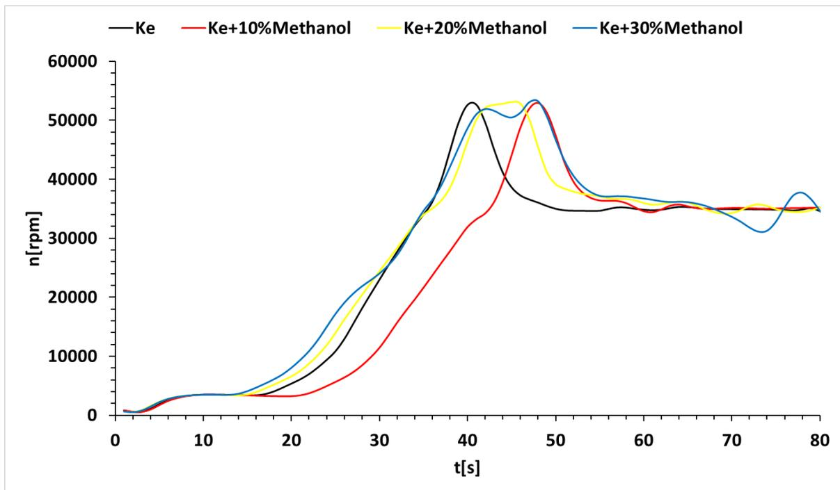
Figure 5. The rpm variation over time during the startup procedure until a stable output is attained.
