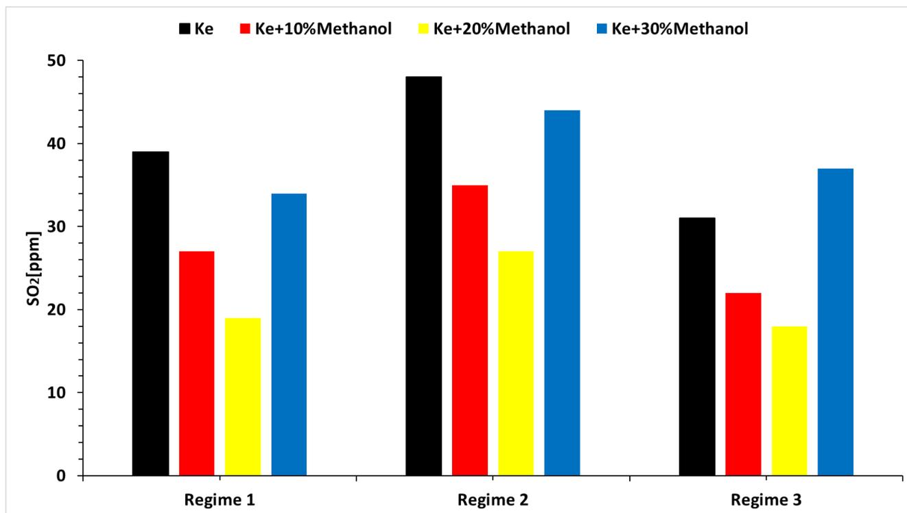
Figure 15. Concentration of SO<sub>2</sub> versus operational modes and fuel blends.
