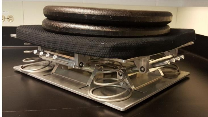
**Figure 5.** The internal mechanism of the novel quasi-zero stiffness cushion with a foam pad on top.
