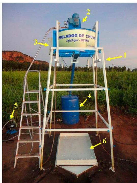
**Figure 1.** Description of the components of the *InfiAsper* rainfall simulator (Legend: metallic structure (1); water application unit (2); control panel (3); water reservoir (4); water pump (5); and runoff collector (6)).
