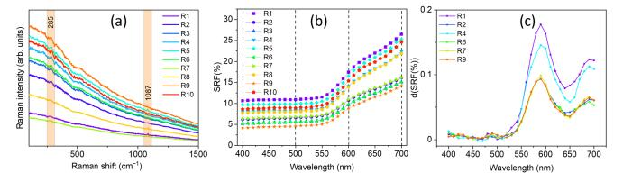
In Figure 5 the obtained portable Raman spectra (Figure 5a), SRF% trends (Figure 5b), and calculated first derivate curves (Figure 5c) are reported, the latter obtained only for five representative red pigmented areas, lighter and darker, respectively.
