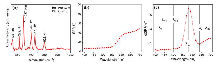
**Figure 2.** (a) Portable Raman spectrum, (b) spectral reflectance factor (SRF%), and (c) d(SRF(%)) curve obtained for sample ID code 11300—*Red jasper*.
