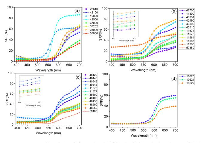
*powder*, 37202—*Madder lake*, 36020—*Lac dye*, and 37030—*Resina kamala*) ranging from 610 nm in the case of sample 42100—*carmine nacarat* to 640 nm for sample 37000—*Dragon's blood*.
