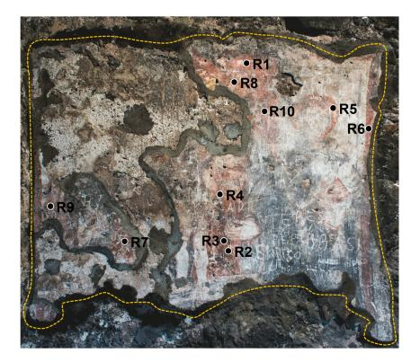
**Figure 1.** Investigated polychrome wall painting located within The Norman Castle of Aci Castello (Catania, Italy), with an indication of the analyzed areas. The yellow-dashed line indicates the painted area. The surface area is  $\sim 2 \text{ m}^2$ .
