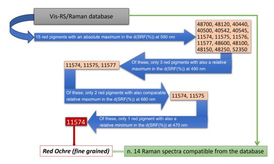
**Figure 6.** Flowchart utilized for the red pigment identification. Blue and green arrows refer, respectively, to vis-RS and portable Raman data.
