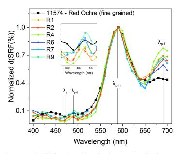
**Figure 7.** d(SRF(%)) vs.  $\lambda$  profiles related to the selected red areas and sample ID code 11574 (taken from the library), with the positions of the  $\lambda_{p-h}$ ,  $\lambda_{p-l}$ , and  $\lambda_v$  features indicated. All curves were normalized to the 590 nm absolute maximum value for a better comparison.
