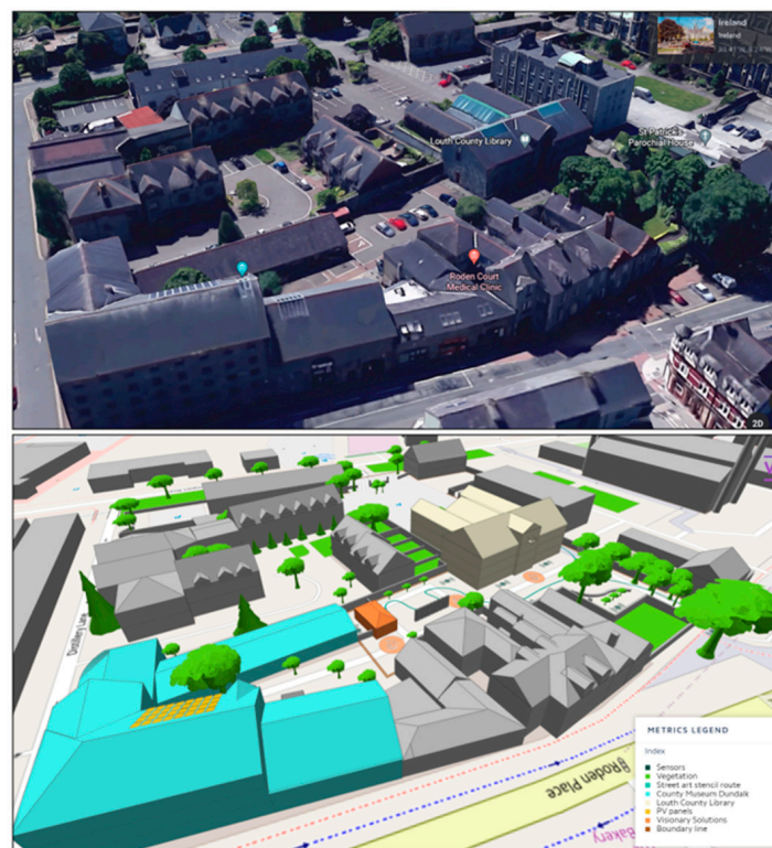
Figure 13. Dundalk digital twin example: Google Earth above, IES digital twin below.
