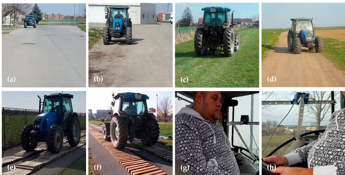
Figure 2. Exploitation measuring on the following: (a) asphalt; (b) gravel; (c) grass; (d) dirt road; (e) rough track; (f) smooth track; with (g) microphone on left side; (h) microphone on right side.
