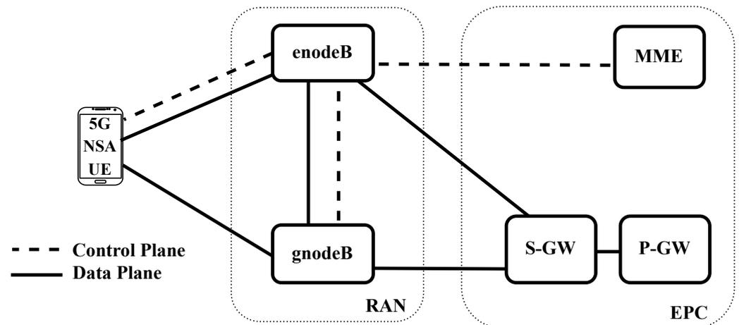
**Figure 1.** The 5G NSA architecture consists of a 4G core network and two types of base stations (BSs).
