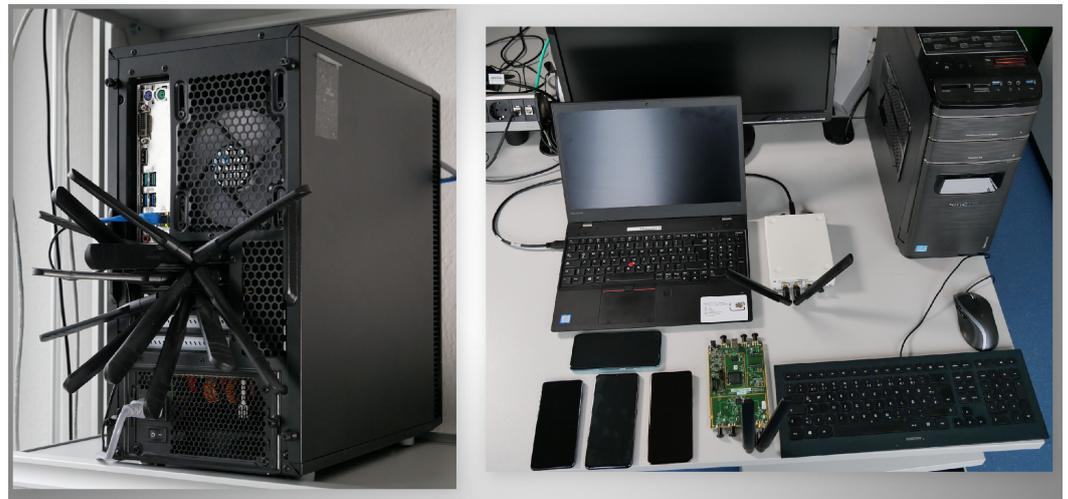
**Figure 5.** Our experimental testbed consisting of an Amarisoft Call Box Classic (left), two SDRs, two personal computers (PCs), test SIM cards, and Commercial Off-the-Shelf (COTS) UE (right).
