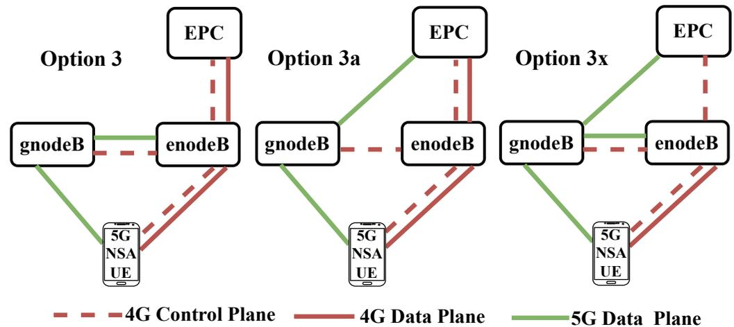
Figure 2. 5G NSA option 3 consists of three variants, namely 3, 3a, and 3x [16].
