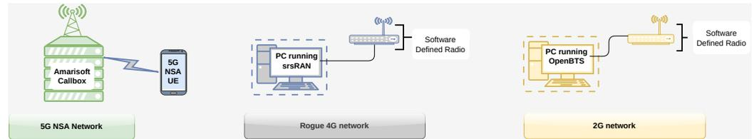
**Figure 4.** Schematic representation of the implemented experimental testbed, featuring a 5G NSA network, a 5G NSA UE, a fake 4G network, and a 2G network.
