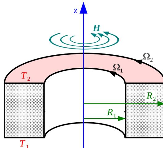
**Figure 9.** An electrically conductive nanofluid fills a layer between two rotating cylinders with angular velocities  $\Omega_1$  and  $\Omega_2$  and is located in a spiral magnetic field. The lower surface of the layer has a temperature of  $T_1$ , the upper surface has a temperature of  $T_2$ , and  $T_1 > T_2$ .
