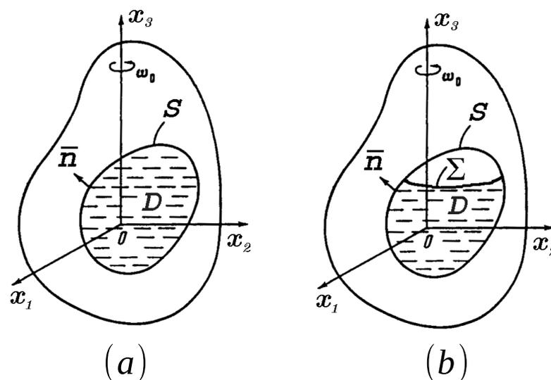
**Figure 1.** Rotating bodies with liquid in cavity ( $D$ ) completely (a) and partially (b) filled; in the latter case, free surface  $\Sigma$  appears.
