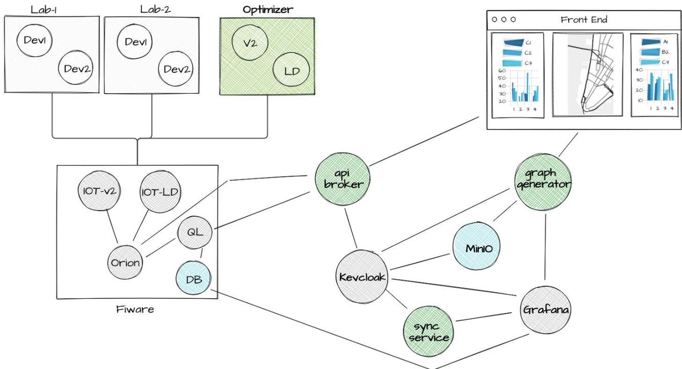
**Figure 1.** The overall architecture; the developed services are highlighted in green. Image drawn with MockFlow (<https://mockflow.com/>).
