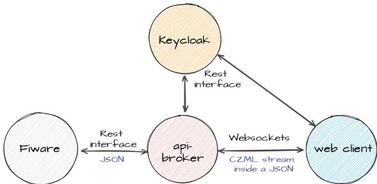
**Figure 11.** The data flow, from FIWARE to Cesium. Image drawn with MockFlow (<https://mockflow.com/>).
