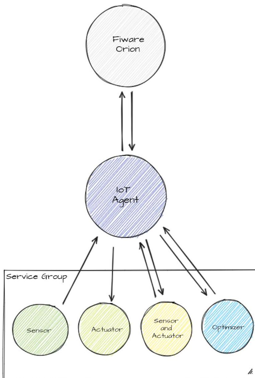
**Figure 15.** Overall architecture of FIWARE Orion, IoT agent, and devices. Image drawn with MockFlow (<https://mockflow.com/>).
