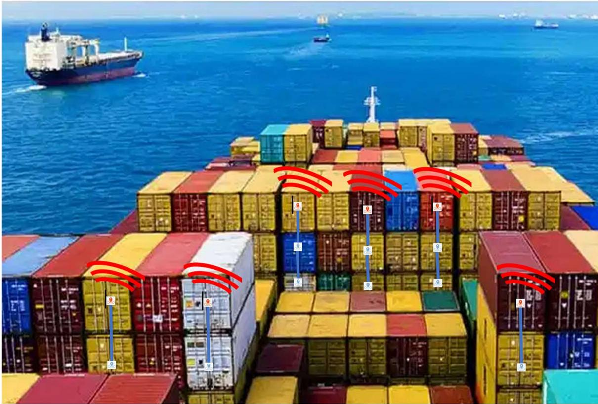
**Figure 3.** Representation of CTDs on the ship: devices at the top of the container stack perform as the NB-IoT/BLE Mesh Gateway, and those below are nodes of BLE Meshes.
