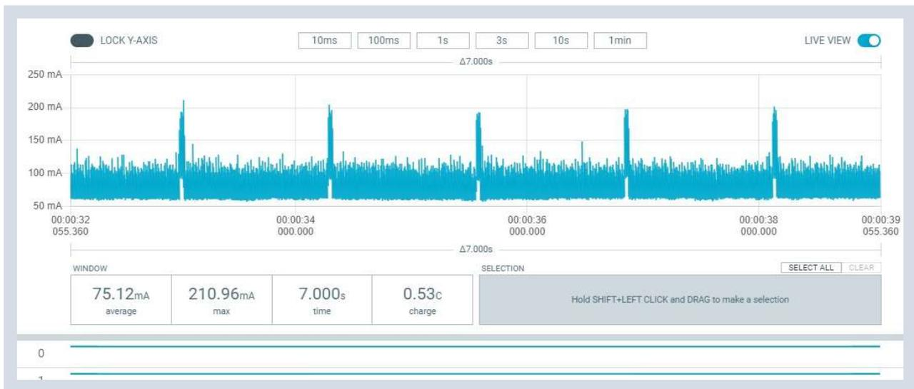
**Figure 18.** Current consumption without sensors ESP32 in active mode with BLE turned on, transmitting periodical beacons [36].
