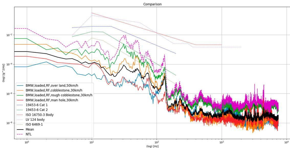
**Figure 7.** Road surfaces: BMW i3/loaded/right front (RF).
