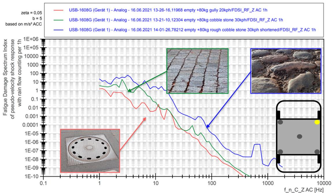
**Figure 6.** FDS for driving over different surfaces for the VW ID.3, calculated for 1h.
