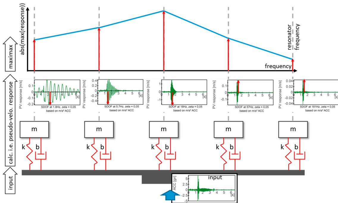
**Figure 5.** Shock Response Spectrum (SRS) calculation for a simplified graph with only five possible resonating frequencies considered.
