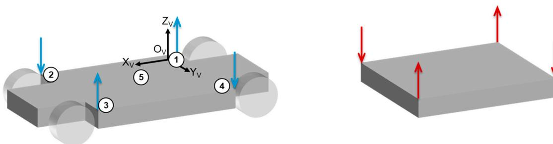
**Figure 2.** Incoherent movements (**left**) and incoherent excitation forces (**right**) on the corners (indicated by different directions) on a vehicle chassis.
