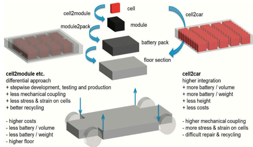
**Figure 1.** Concepts of cell2car and module2pack [1].
