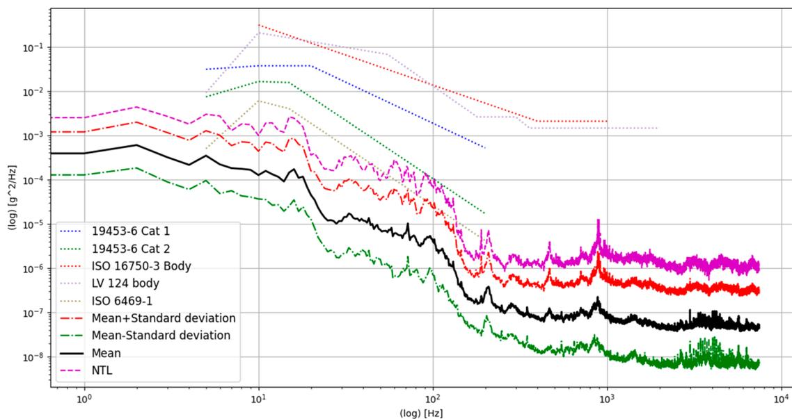
Figure 9. Statistical evaluation of the VW ID.3 over all measurement data.
