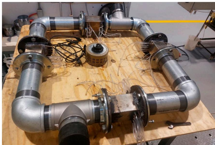
Figure 3. Traveling-wave thermo-acoustic electricity generator.
