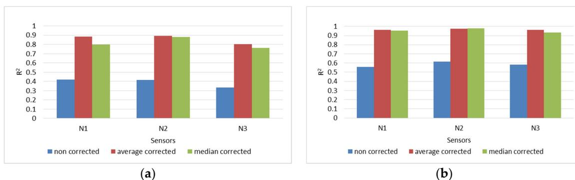
**Figure 26.** LR correlations ( $R^2$ ) of non-corrected, corrected by average method, and corrected by median method, measurements in respect to the reference measurements. (a) LR correlations ( $R^2$ ) of  $\text{NO}_2$  gas concentrations, (b) LR correlations ( $R^2$ ) of  $\text{O}_3$  gas concentrations.
