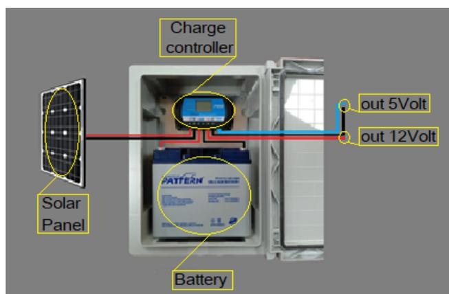
**Figure 3.** Autonomous power supply.
