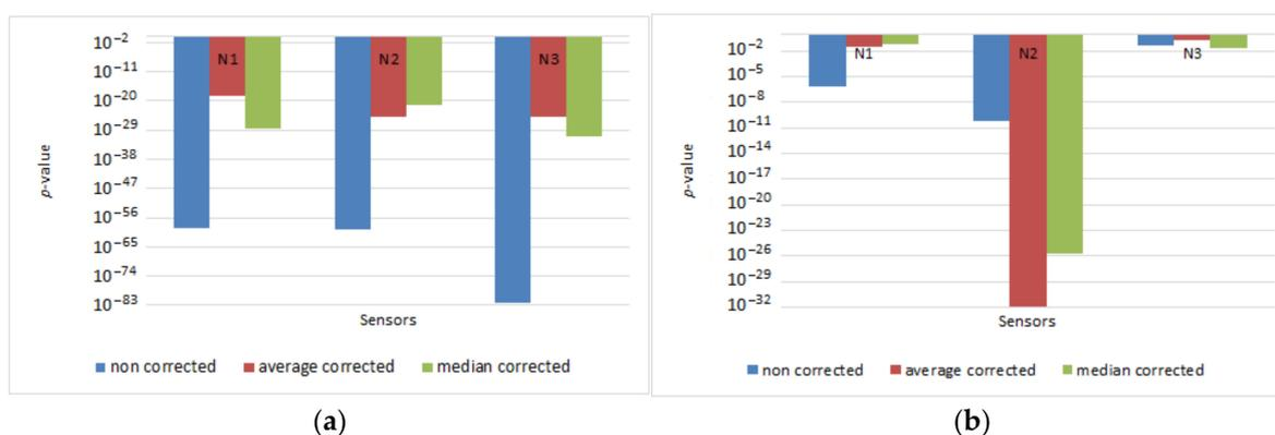
**Figure 27.** Value of LR interception ( $p$ -value) of non-corrected, corrected by average method, and corrected by median method, measurements in respect to the reference measurements. (a) LR interception ( $p$ -value) of  $\text{NO}_2$  gas concentrations, (b) LR interception ( $p$ -value) of  $\text{O}_3$  gas concentrations.
