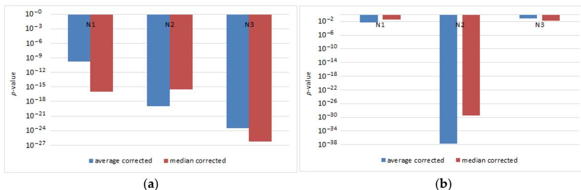
**Figure 29.** Value of MLR interception ( $p$ -value) corrected by average method and corrected by median method, measurements in respect to the reference measurements. (a) MLR intercept ( $p$ -value) of NO<sub>2</sub> gas concentrations, (b) MLR interception ( $p$ -value) of O<sub>3</sub> gas concentrations.
