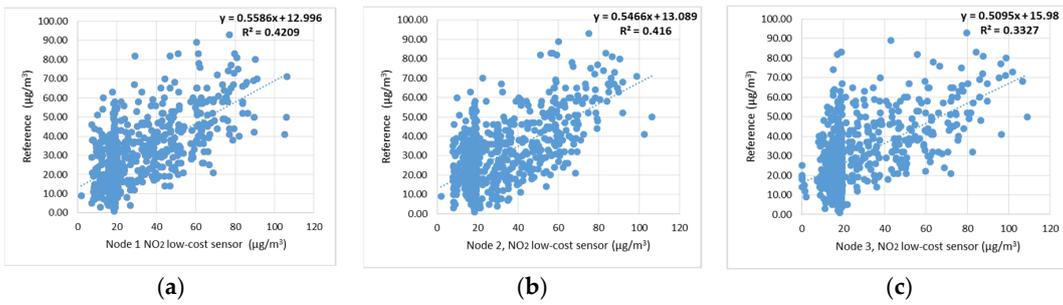
Figure 7. Scatter plot of values of each LCS NO<sub>2</sub> (N1, N2, N3) and reference. (a) Scatter plot of measurements of Node 1 NO<sub>2</sub> LCS and reference, (b) Scatter plot of measurements of Node 2 NO<sub>2</sub> LCS and reference, (c) Scatter plot of measurements of Node 3 NO<sub>2</sub> LCS and reference.
