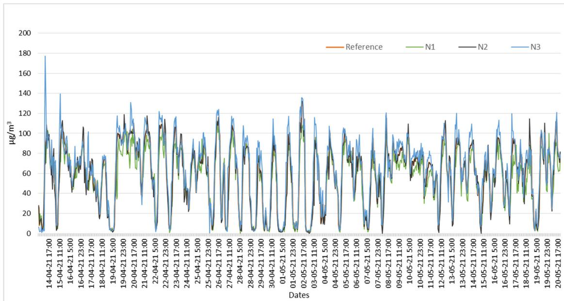
**Figure 24.** Corrected values of each low-cost O<sub>3</sub> sensor using the median variation as correction factor in relation to the reference values.
