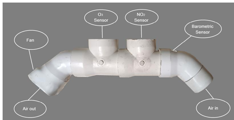
**Figure 5.** Sensor holder tube.
