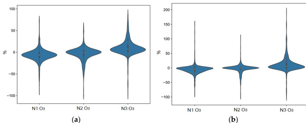
**Figure 17.** Violin curves of O<sub>3</sub> LCS. (a) Percentage change distribution of average method of O<sub>3</sub> measurements. (b) Percentage change distribution of median method of O<sub>3</sub> measurements.
