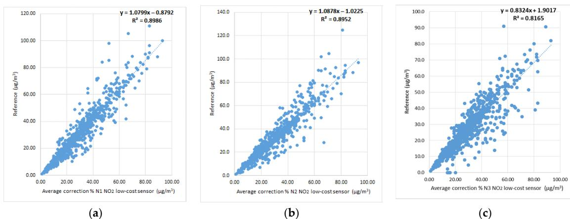
**Figure 19.** Scatter plots of corrected values (average variation) in relation to the reference values of each  $NO_2$  sensor. (a) Scatter plot of corrected values in relation to the reference values of  $NO_2$  sensor of Node 1. (b) Scatter plot of corrected values in relation to the reference values of  $NO_2$  sensor of Node 2. (c) Scatter plot of corrected values in relation to the reference values of  $NO_2$  sensor of Node 3.
