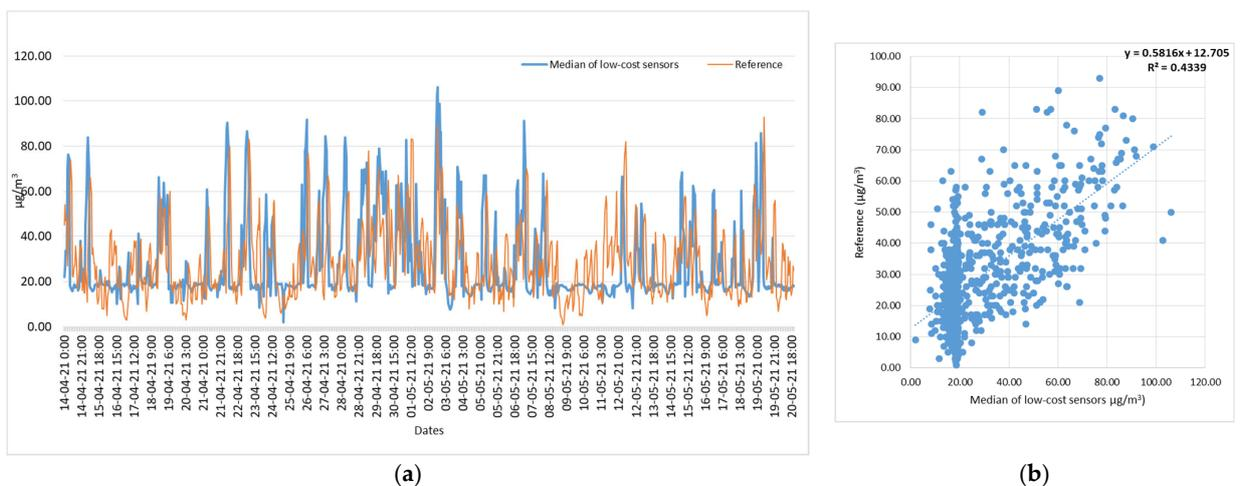
**Figure 11.** Performance of median values of three low-cost nitrogen dioxide sensors and the reference values. (a) Time series of the median values and reference values of nitrogen dioxide concentration, (b) Scatter plot between the median and reference values of nitrogen dioxide concentration.
