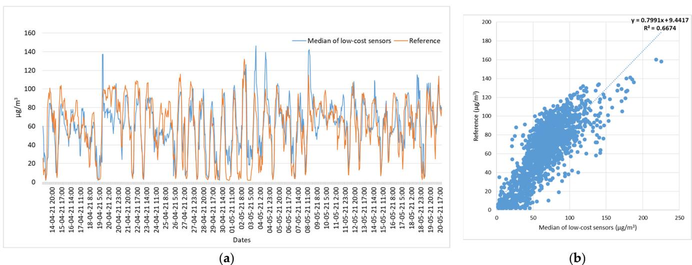
**Figure 13.** Performance of median values of three low-cost ozone sensors and the reference values. (a) Time series of the median values and reference values of ozone concentration, (b) Correlation ( $R^2$ ) between the median and reference values of ozone concentration.
