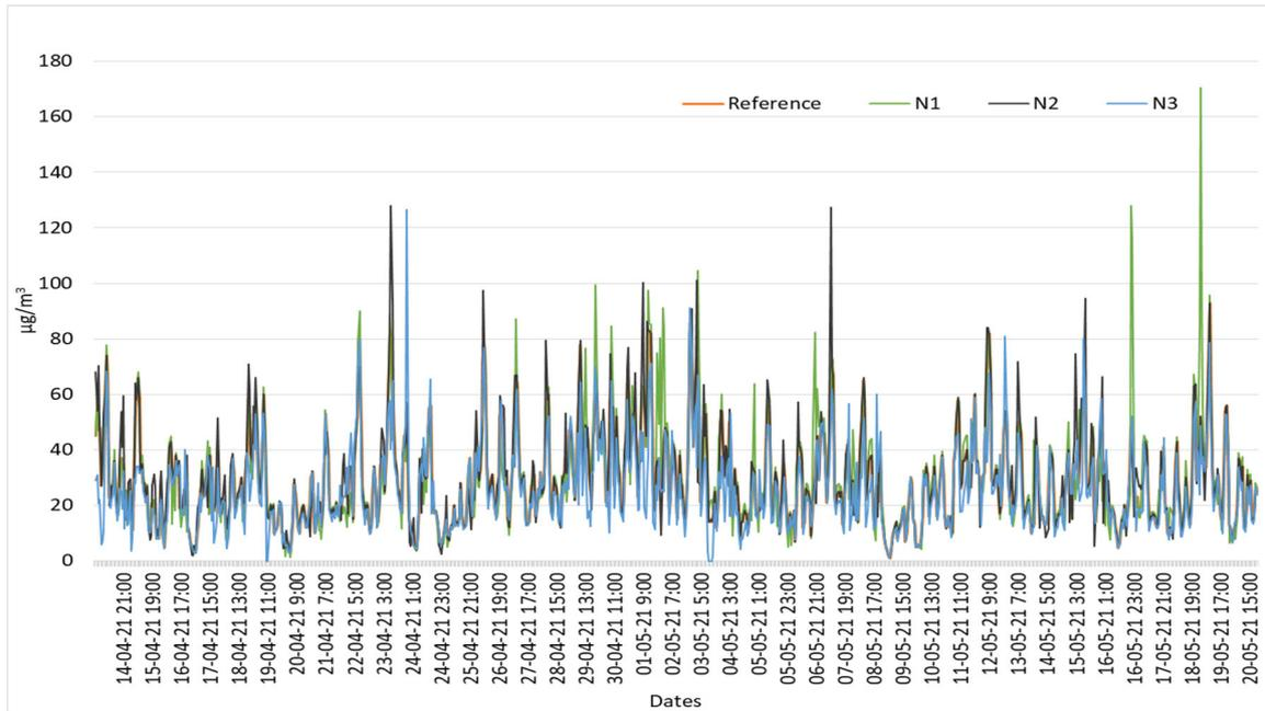
**Figure 20.** Corrected values of each low-cost NO<sub>2</sub> sensor using the median variation as correction factor in relation to the reference values.
