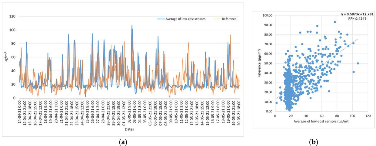
**Figure 10.** Performance of average values of three low-cost nitrogen dioxide sensors and the reference values. (a) Time series of the average values and reference values of nitrogen dioxide concentration, (b) Scatter plot between the average and reference values of nitrogen dioxide concentration.
