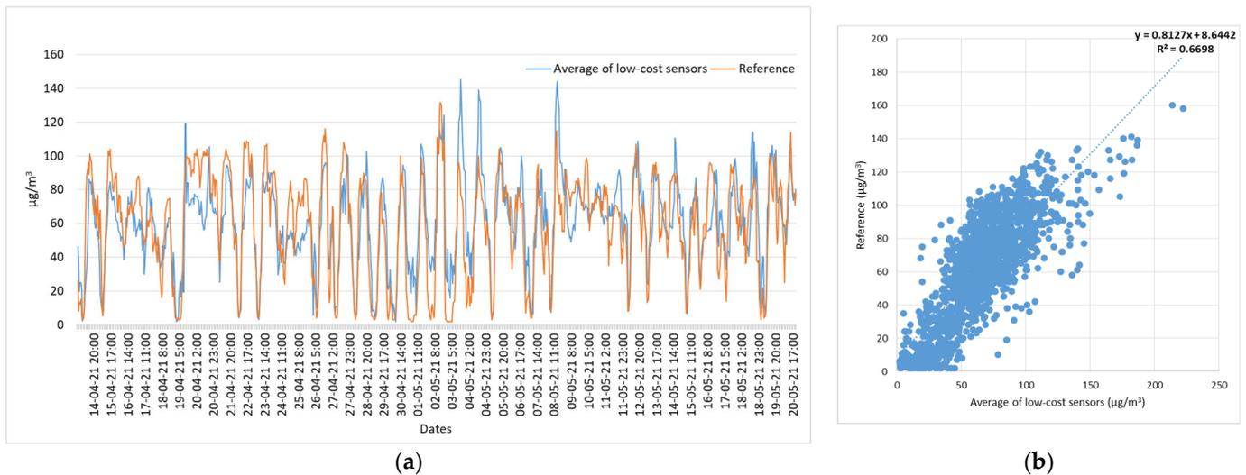
**Figure 12.** Performance of average values of three low-cost ozone sensors and the reference values. (a) Time series of the average values and reference values of ozone concentration, (b) Correlation ( $R^2$ ) between the average and reference values of ozone concentration.
