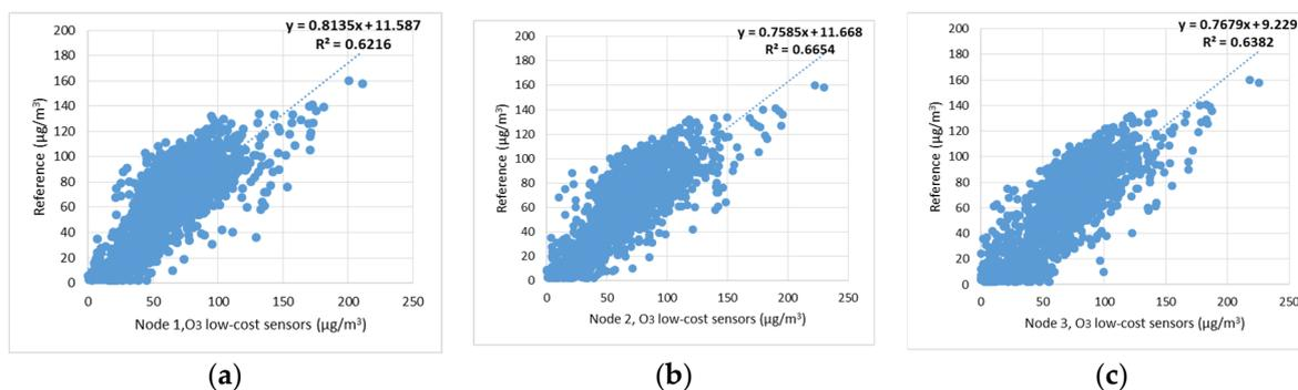
**Figure 9.** Scatter plot of values of each LCS O<sub>3</sub> (N1, N2, N3) and reference. (a) Scatter plot of measurements of Node 1 O<sub>3</sub> LCS and reference, (b) Scatter plot of measurements of Node 2 O<sub>3</sub> LCS and reference, (c) Scatter plot of measurements of Node 3 O<sub>3</sub> LCS and reference.
