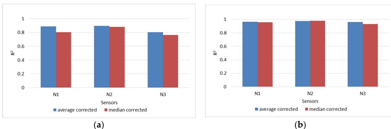
**Figure 28.** MLR correlations ( $R^2$ ) of corrected by average method and corrected by median method, measurements in respect to the reference measurements. (a) MLR correlations ( $R^2$ ) of NO<sub>2</sub> gas concentrations, (b) MLR correlations ( $R^2$ ) of O<sub>3</sub> gas concentrations.
