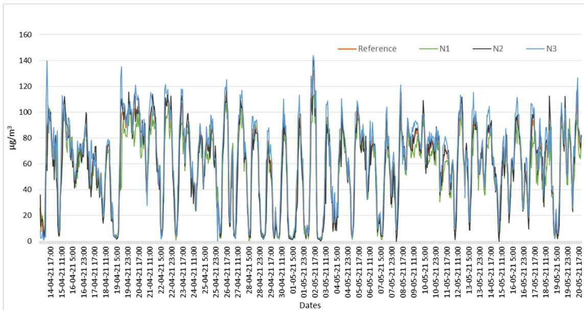
**Figure 22.** Corrected values of each low-cost O<sub>3</sub> sensor using the average variation as correction factor in relation to the reference values.
