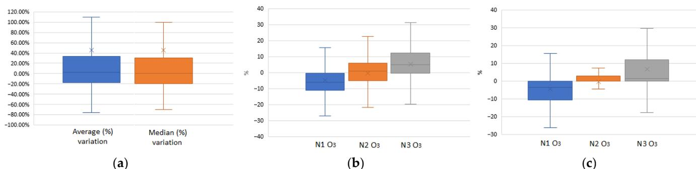
**Figure 15.** Boxplots of O<sub>3</sub> LCS. (a) Total variation including the values of all three low-cost O<sub>3</sub> sensors, both the average and the median. (b) Variation of each low-cost O<sub>3</sub> sensor in relation to the percentage average values and reference values for each sensor. (c) Variance of each low-cost O<sub>3</sub> sensor in relation to the median average variance values versus the reference values for each sensor.
