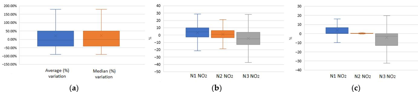
**Figure 14.** Boxplots of NO<sub>2</sub> LCS. (a) Total variation including the values of all three low-cost NO<sub>2</sub> sensors, both the average and the median. (b) Variation of each low-cost NO<sub>2</sub> sensor in relation to the percentage average values and reference values for each sensor. (c) Variation of each low-cost NO<sub>2</sub> sensor in relation to the percentage median values and reference values for each sensor.
