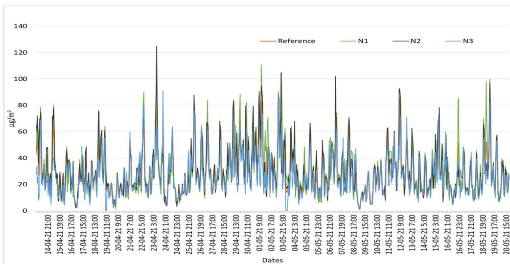
**Figure 18.** Corrected values of each low-cost  $NO_2$  sensor using the average variation as correction factor in relation to the reference values.
