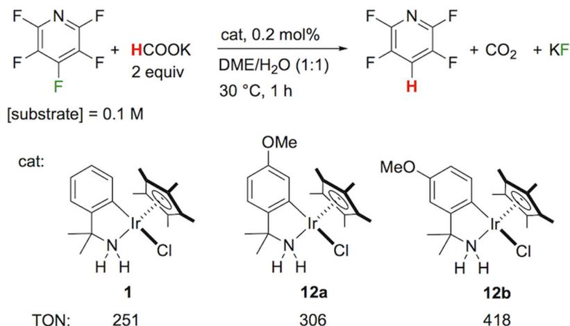
**Scheme 6.** Comparison of the catalytic activities of **1**, **12a**, and **12b** for the transfer hydrogenative defluorination of pentafluoropyridine with HCOOK.
