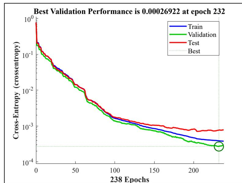
**Figure 3.** The resulted cross-entropy from training process for the PR-NN model.
