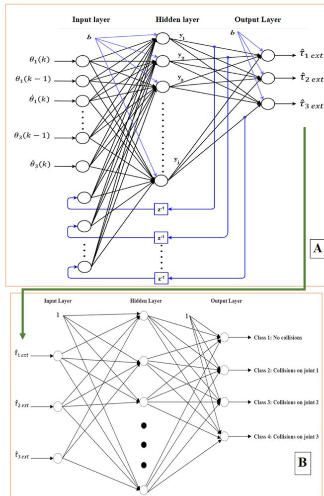
**Figure 1.** The proposed method to create a PR-NN classifier model: (A) The structure of the trained RNN used to estimate the external torques on joints; (B) The proposed PR-NN model which classifies collision according to its inputs of estimated external torques.
