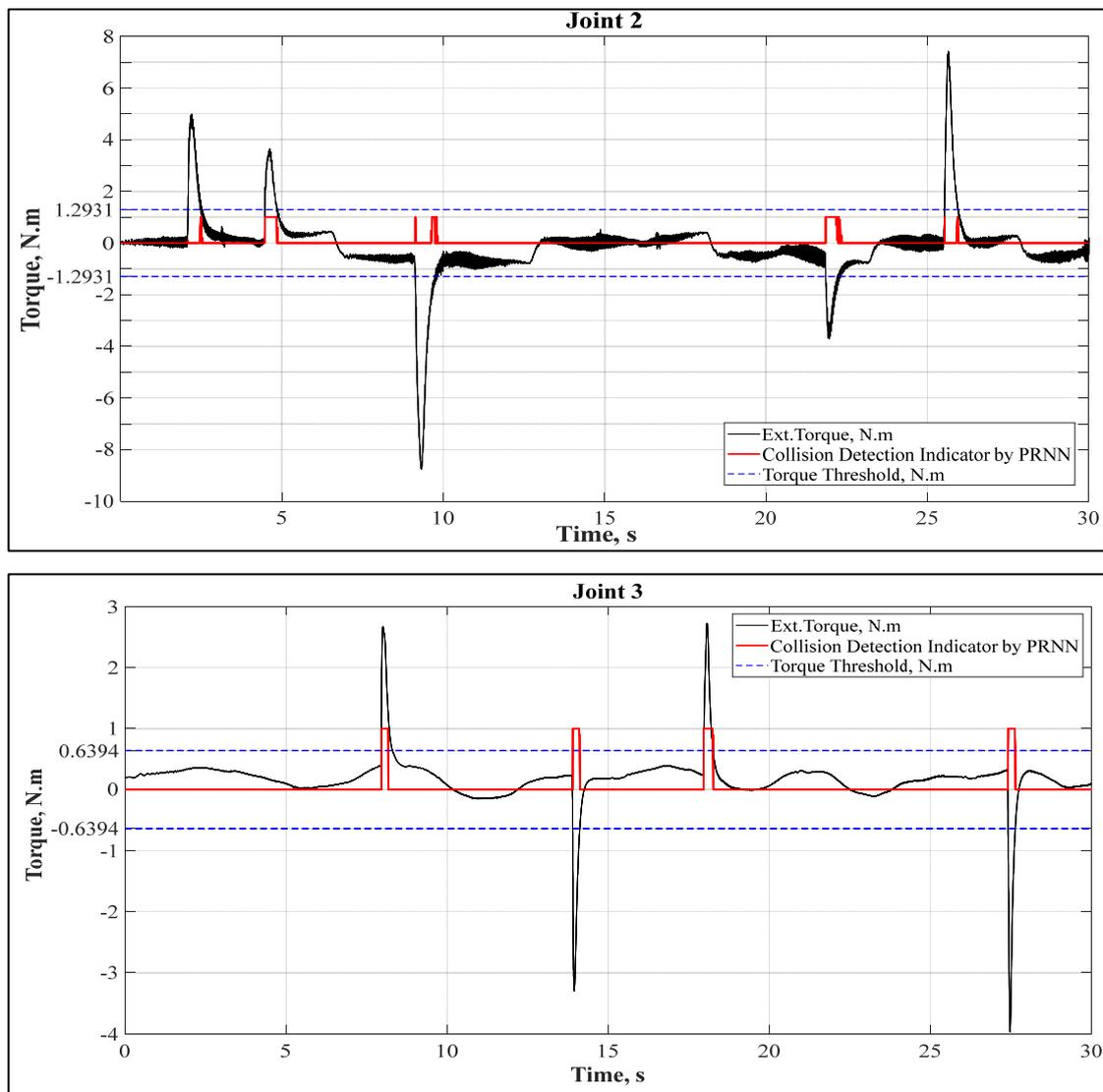
**Figure 8.** Response of the PR-NN classifier model to the torque signals exerted on the joints.
