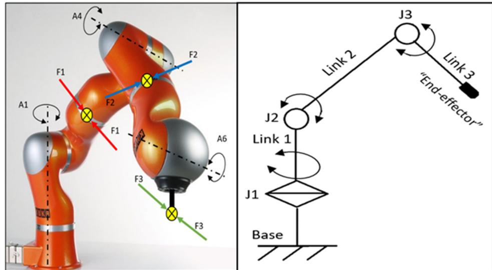
**Figure 2.** Configuration of the KUKA robot as a 3-DOF robot and direction of applying collisions.
