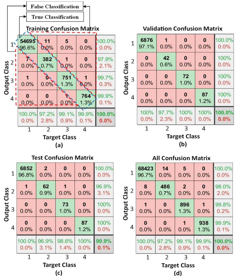
**Figure 7.** Confusion matrices showing the effectiveness of the PR-NN model during (a) the training process, (b) the validation process, (c) the testing process, and (d) when all collected data are used to train the PR-NN model. Four classes are presented in the confusion matrices: Class (1): No collisions, Class (2): Collision on Link 1, Class (3): Collision on Link 2, Class (4): collision on Link 3.
