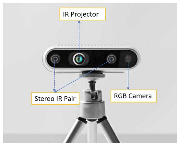
**Figure 2.** Intel RealSense depth camera D435.
