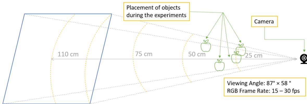
**Figure 5.** Experimental setup and locations of different objects during the experiment.
