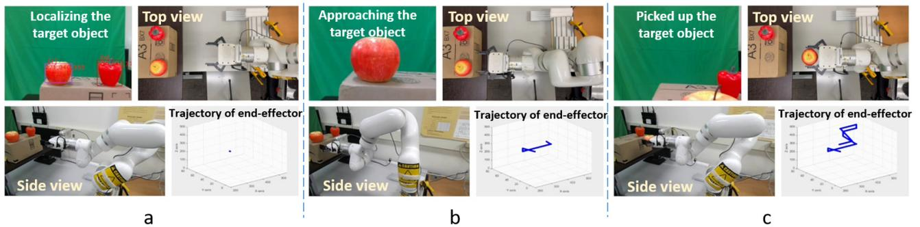
**Figure 7.** System performance from three different viewpoints, along with the end-effector's position during an experiment: (a) at the beginning of the experiment, (b) in the middle of the experiment, and (c) at the end of the experiment.
