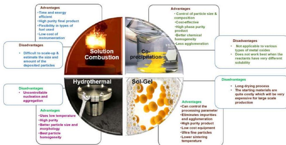
**Figure 19.** Schematic showing the advantages and disadvantages of the most widely used wet-chemical routes.
