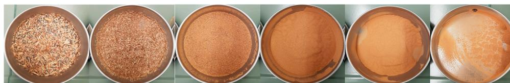
**Figure 3.** The sieves, from left to right: 2000, 630, 200, 112, and 63  $\mu\text{m}$ , and the sieve base with sawdust fractioned by electric sieve-shaker.
