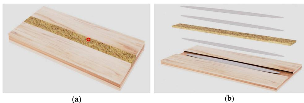
**Figure 1.** (a) The bottom side of laminated plywood with a composite of eucalyptol–sawdust filling the slit and a 0.8 mm aperture in the dry PVA layer. (b) The bottom side of laminated plywood with two layers of PVA glue in the groove/slit, then the composite of eucalyptol–sawdust, and two layers of PVA glue on the composite.
