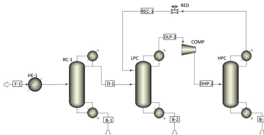
**Figure 1.** Process scheme used for the simulations of EtOH distillation, adapted from Karimi et al. [7].
