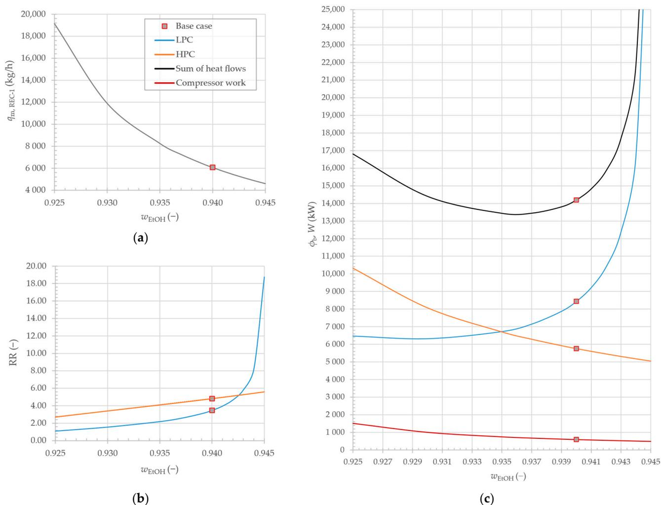
**Figure 7.** The effect of EtOH fraction in the distillate of LPC on (a) mass flow rate of recycle REC-1; (b) RR of distillation columns; (c) boiler heat demand and necessary compressor work.
