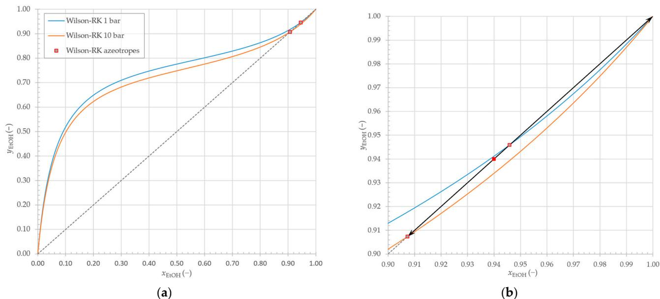
**Figure 2.** (a) EtOH-H<sub>2</sub>O xy diagram; (b) EtOH-H<sub>2</sub>O xy diagram magnified at the location of azeotrope shift (full red square shows EtOH fraction of distillate, achieved in LPC, while the black line shows the possible operation of HPC).
