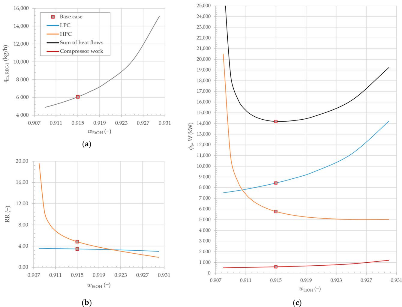
**Figure 8.** The effect of EtOH fraction in distillate of HPC on (a) mass flow rate of recycle REC-1; (b) RR of distillation columns; and (c) boiler heat demand and necessary compressor work.
