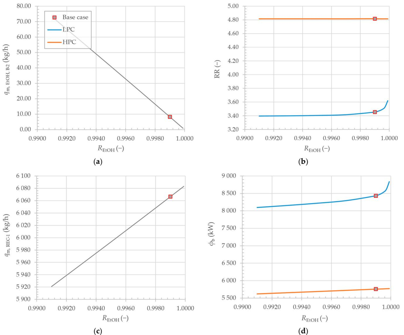
**Figure 6.** The effect of EtOH recovery on: (a) losses of EtOH in distillation bottom B-2; (b) RR of distillation columns; (c) mass flow of REC-1; and (d) heat demand in distillation column boilers.
