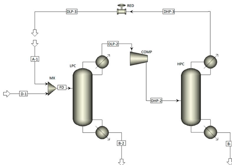
**Figure 3.** Initial process scheme for the simulation of PSD.
