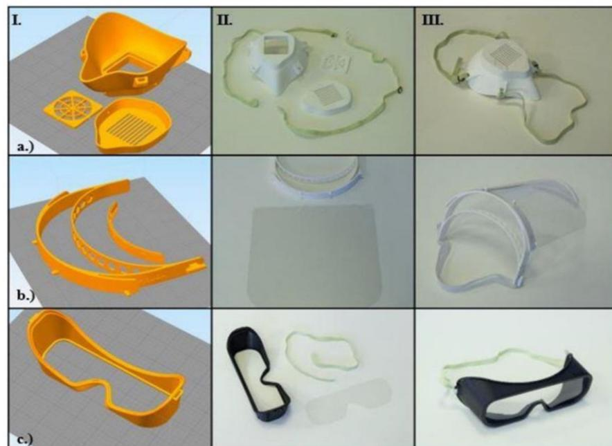
**Figure 1.** Overview of personal protective equipment (PPE) manufacturing process using 3D printing. With Column I—demonstrating CAD assembly, II—3D printed parts, III—the assembled models. The rows show (a) a respirator face mask; (b) a face shield; (c) a pair of safety goggles. This image is reprinted under a Creative Commons Attribution 4.0 International License and it is taken from [18].
