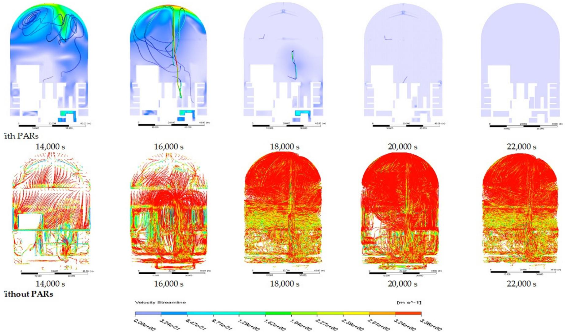
Figure 9. Comparison of velocity streamlines in containments with and without PARs as a function of time.
