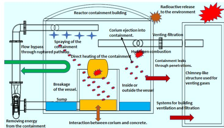
**Figure 1.** Main physical phenomena during a severe accident.
