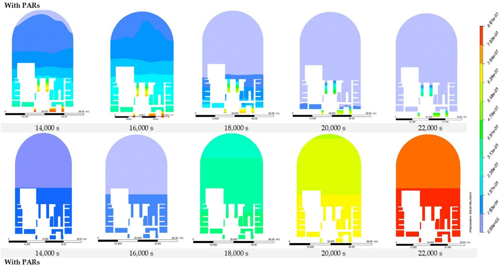
Figure 8. Pressure distributions in containment models with and without PARs as a function of time.
