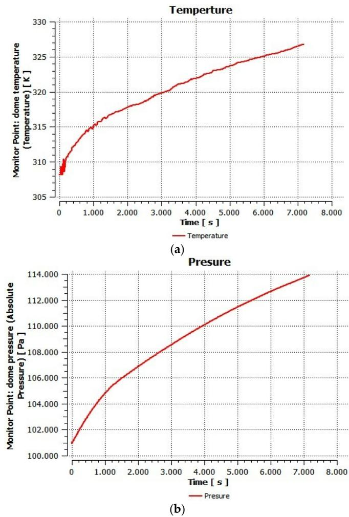
Figure 4. (a) Dome temperature as a function of time; (b) dome pressure as a function of time.
