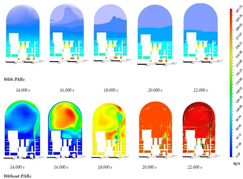
Figure 5. Comparison of hydrogen distributed during the test with and without PARs as a function of time.
