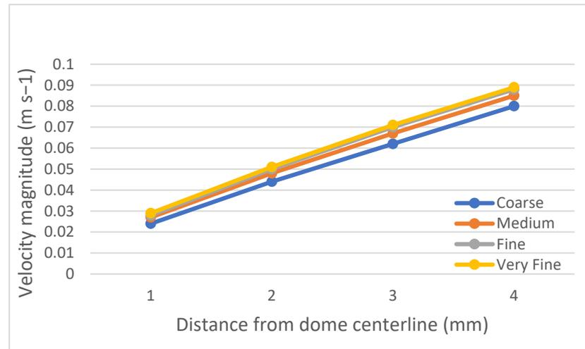
Figure 3. Grid independence study of different mesh distributions.
