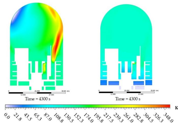
**Figure 7.** Snapshots of mass flow concentrations of hydrogen distributed in the containments with (right) and without (left) PARs.
