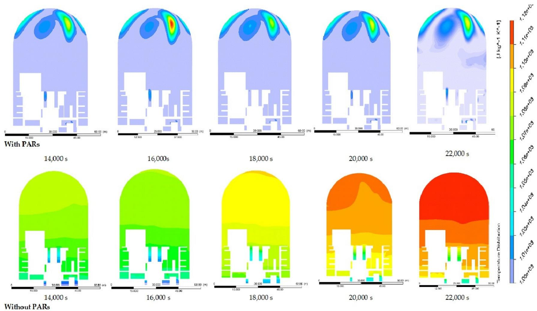
Figure 6. Comparison of temperature distributed during the tests for containments with and without PARs as a function of time.
