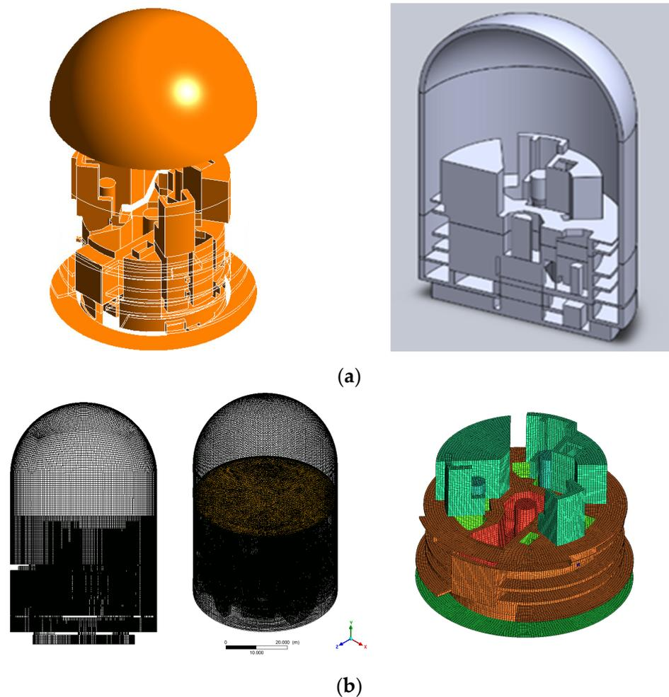
**Figure 2.** (a) Three-dimensional containment model. (b) Mesh of the 3D containment model.
