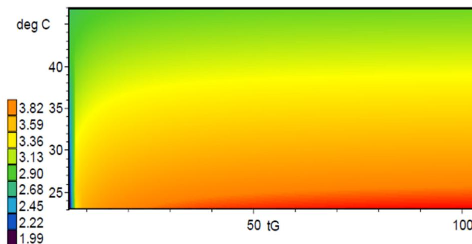
**Figure 5.** The 2D resolution map of T versus  $t_G$  generated by DryLab<sup>®</sup>; The best resolution of the critical peak pair is achieved by implementing the conditions offered by the red area of the map, while the blue areas offer the worst resolutions. Colors in between offer various resolution options.
