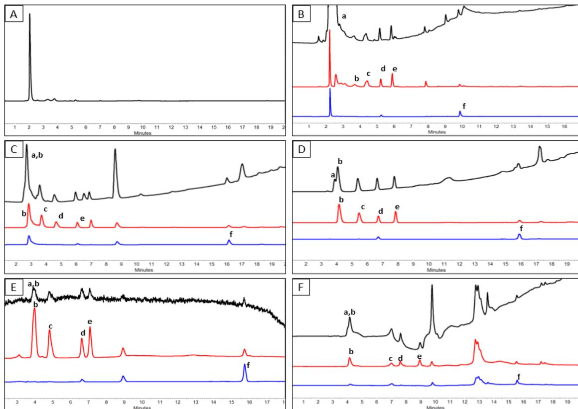
**Figure 3.** (A): Extracted unspiked plasma sample (detector: 266 nm), (B): Experimental chromatogram of extracted plasma sample spiked with the six analytes of interest, (C): Experimental chromatogram
