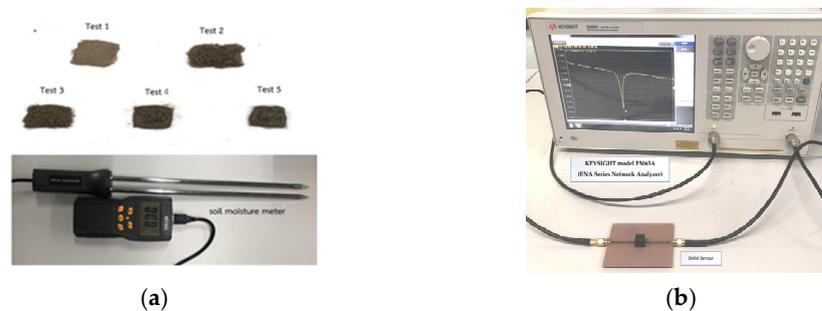
**Figure 4.** The experimental setup; (a) involves various methods for measuring soil moisture; (b) measurement setup.
