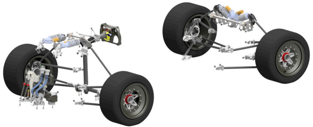
Figure 1. The steering mechanism and suspension model of the ART_X vehicle (the ART's own property).
