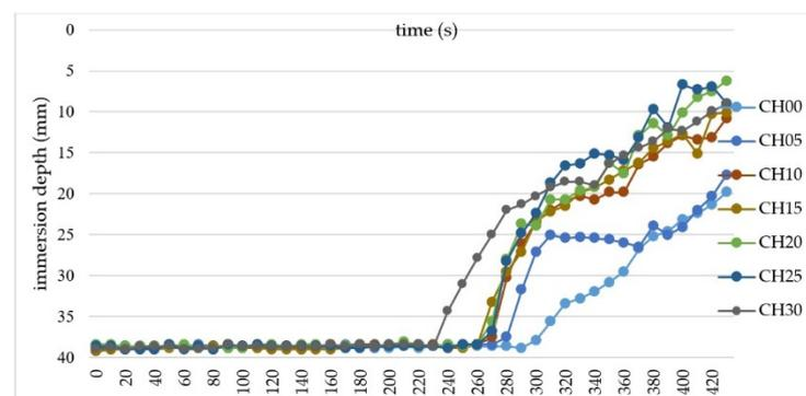
**Figure 2.** Cement-based mortar setting times.
