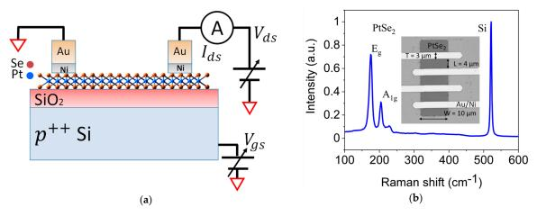
**Figure 1.** (a) Schematic of PtSe<sub>2</sub> back-gated FET and measurement configuration; (b) Raman characterization of PtSe<sub>2</sub> sheet, showing  $E_g$  peak at 176 cm<sup>-1</sup> and  $A_{1g}$  peak at 205 cm<sup>-1</sup>. Inset: SEM image of the device.
