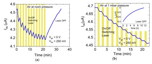
**Figure 3.** (a)  $I_{ds}$  drain current subjected to switching light pulses (30 mW/cm<sup>2</sup>), monitored in air at room pressure. (b)  $I_{ds}$  drain current subjected to switching light pulses (30 mW/cm<sup>2</sup>), monitored in air at  $10^{-3}$  mbar pressure.
