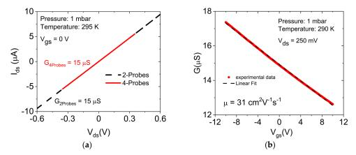
**Figure 2.** (a)  $I_{ds} - V_{ds}$  output curves measured in two- and four-probe configurations. (b)  $G - V_{gs}$  transfer curve showing p-type behaviour and field-effect mobility of 31 cm<sup>2</sup> V<sup>1</sup> s<sup>-1</sup>.
