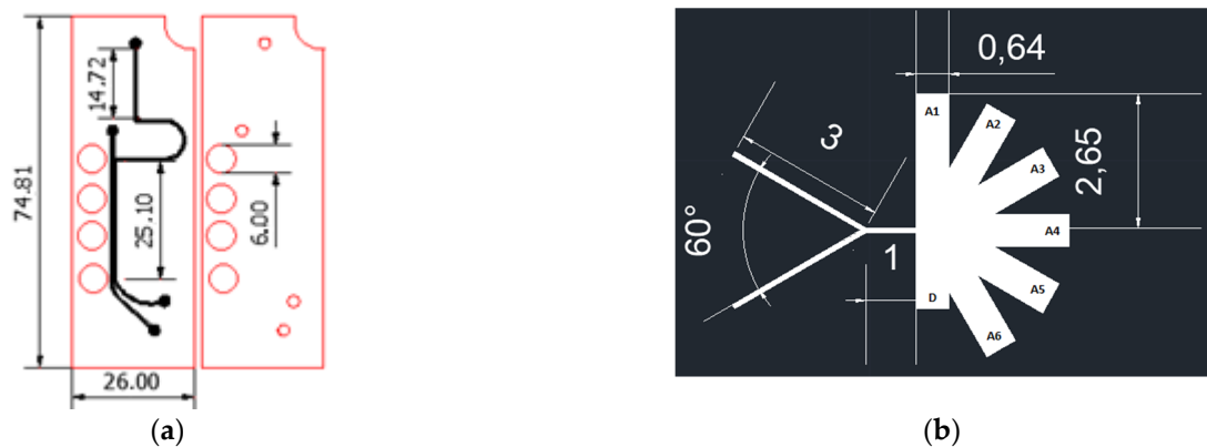
Figure 1. Separation microfluidic system designs (dimensions in mm) (a) Magnetic separation microfluidic system; (b) AsPFF separation microfluidic system.
