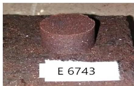
Figure 9. Peridotite sample E6743 without additives after calcination.
