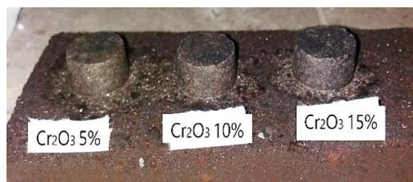
Figure 8. Peridotite E6382 with the Cr<sub>2</sub>O<sub>3</sub> addition after calcination.
