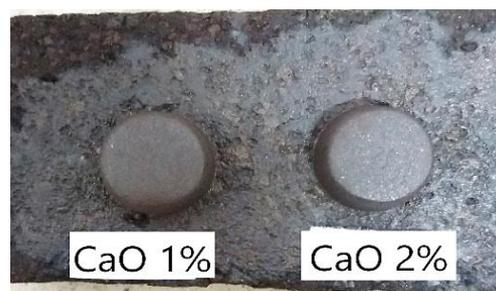
Figure 4. Peridotite sample E6382 with the CaO addition after calcination.
