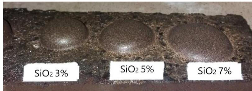
Figure 6. Peridotite sample E6382 with the SiO<sub>2</sub> addition after calcination.
