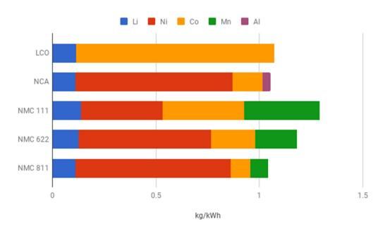
**Figure 2.** Comparison of different battery chemistries, LCO, NCA, and NMC, and their material/elemental composition, according to [6].
