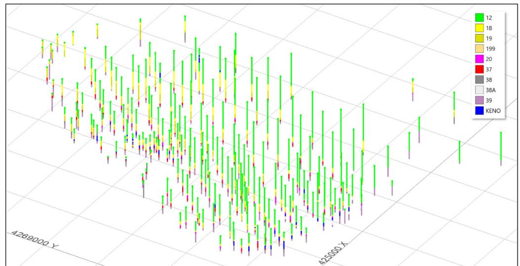
**Figure 2.** Drillholes from the Tsouka deposit coloured by domains with a 100 × 100 m grid overlay.
