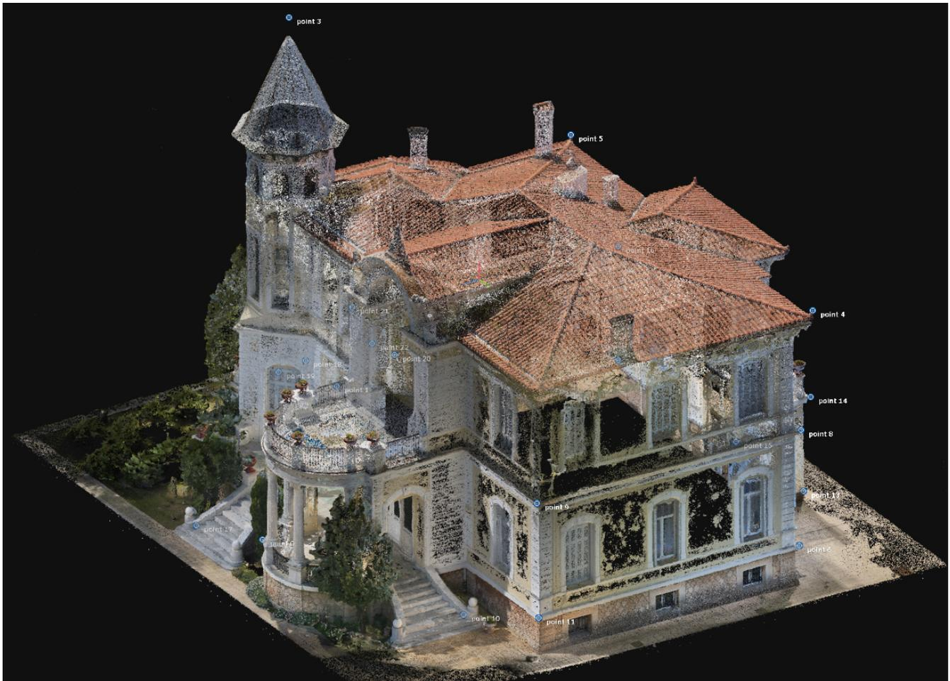
**Figure 8.** Aerial photography registrations and manually inserted ground control points.
