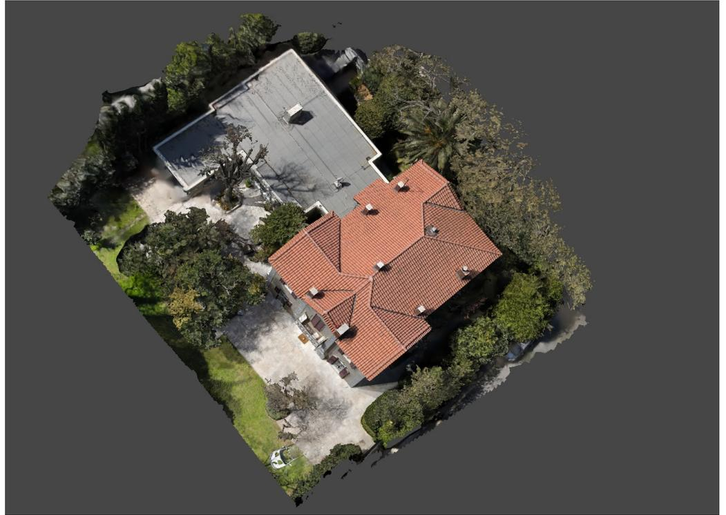
Figure 11. 3D model of a mansion using a drone for aerial photogrammetry.
