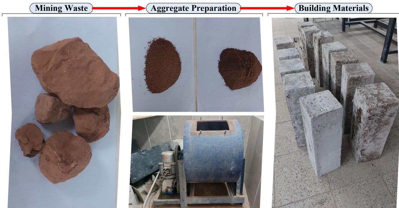
**Figure 2.** The process of utilizing mining waste as building materials.
