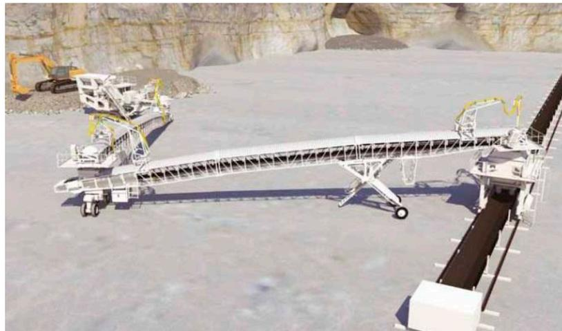
**Figure 7.** Full-Mobile In-pit Crushing and Conveying systems [38] (Source: McCarthy, 2013).
