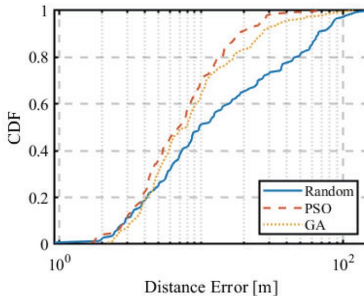
Figure A3. CDF of localization error (optimization algorithm comparison).
