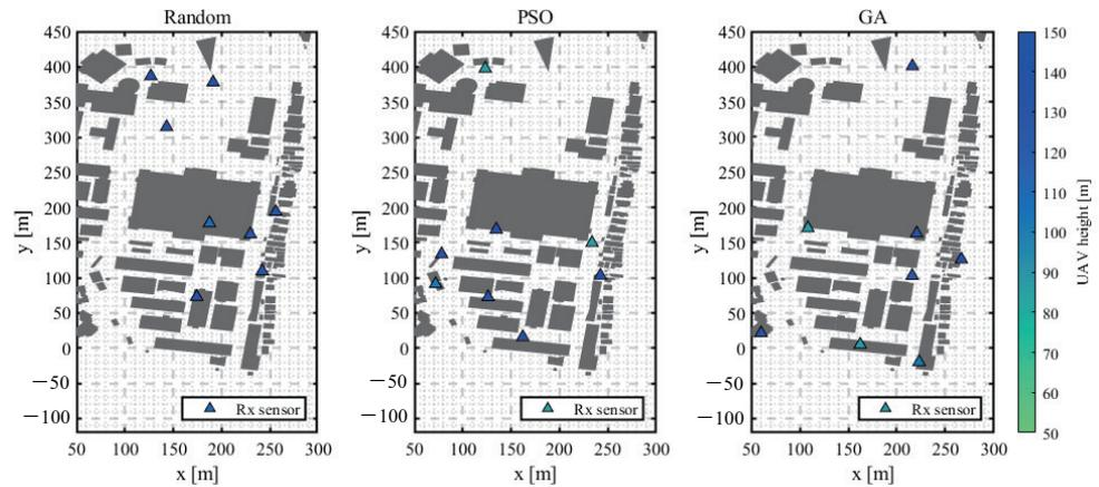
Figure A1. Locations of hovering UAV sensors (optimization algorithm comparison).
