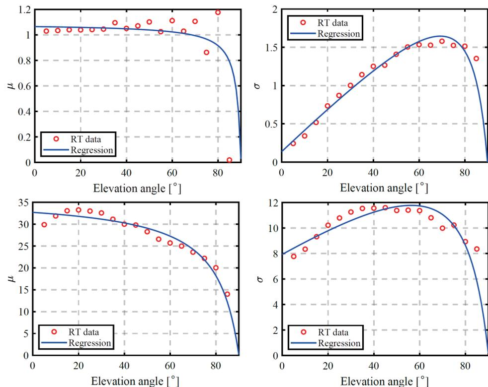
Figure 7. Model parameter determination by regression (top row:  $\mu_n, \sigma_n$  and bottom row:  $\mu_s, \sigma_s$ ).
