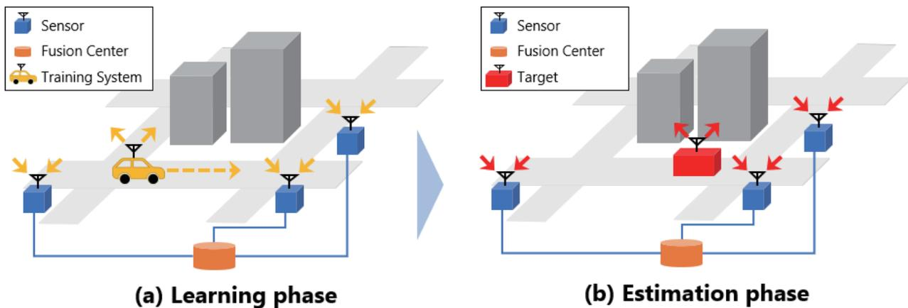
Figure 2. Two phases of fingerprint-based localization method.
