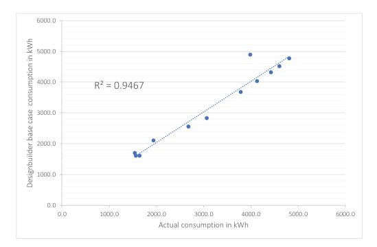
Figure 11. The coefficient of determination between actual and simulated values (R2).
