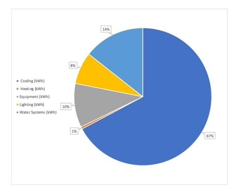
Figure 10. The energy consumption breakdown for the base case.
