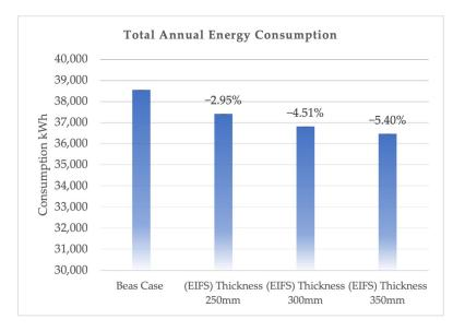
Figure 14. The annual energy performance of utilising different (EIFS) thicknesses for walls.
