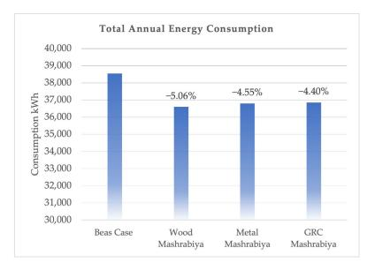
Figure 13. The energy performance of different materials used for Mashrabiya as shading devices.
