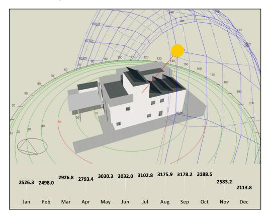
**Figure 15.** Monthly electricity generation (kWh) of one building from PV panels. (T = 34,149.2 kWh/year).
