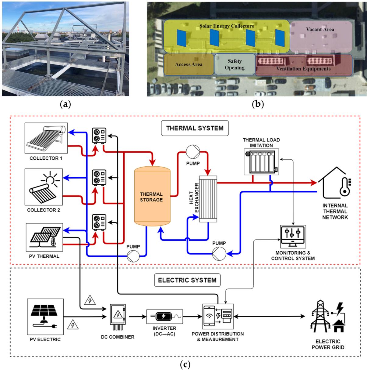
Figure 3. Rooftop view (a) and bird's eye view (b) of the outdoor installation site, and the proposed schematic for the solar energy laboratory (c).
