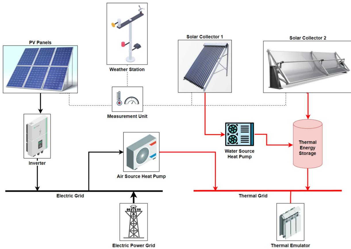
**Figure 2.** Generalized diagram for the proposed solar energy laboratory.
