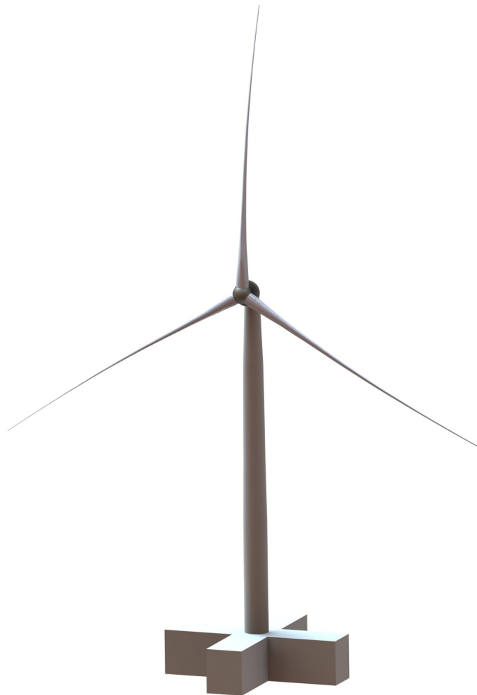
Figure 13. Rendering of the converged platform with the IEA 15-MW turbine.
