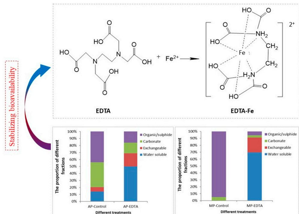
**Figure 8.** The mechanism of adding ligand as an additive to stable bioavailability of trace elements (using Fe as an example). In this picture, the ligand is EDTA and the trace element is Fe. Pictures are drawn from previous published data from Cai et al. [142]. Note: AP means acidogenic phase and MP means methanogenic phase. The water-soluble fraction of trace element has higher bioavailability than other fractions.
