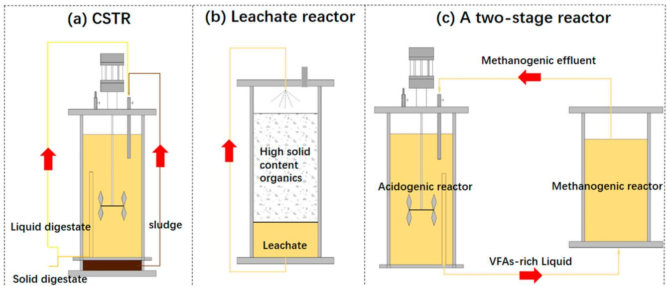
**Figure 3.** Four recirculation types for three common reactors. (a) Liquid digestate or sludge recirculation. (b) Leachate recirculation in leachate reactor with high-solid-content organics as the substrate. (c) The digestate in methanogenic reactor recirculates to acidogenic reactor in a two-stage reactor. The picture was adapted from Zamanzadeh et al. [83] and Pezzolla et al. [81].
