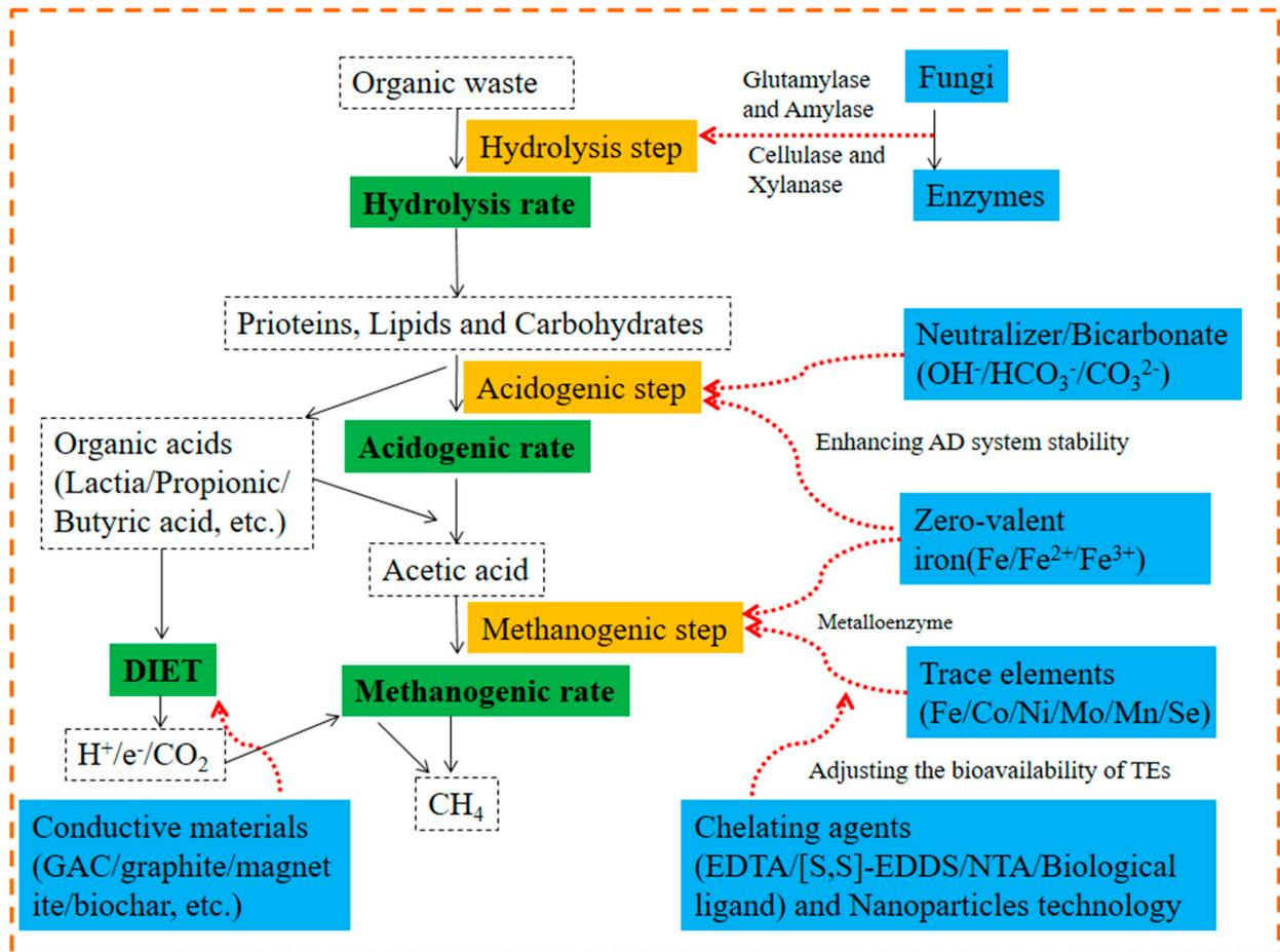
**Figure 5.** The mechanisms of different additives for AD. GAC: Granular Activated Carbon; DIET: direct interspecies electron transfer; TEs: trace elements. This picture was adapted from Ye et al. [109].
