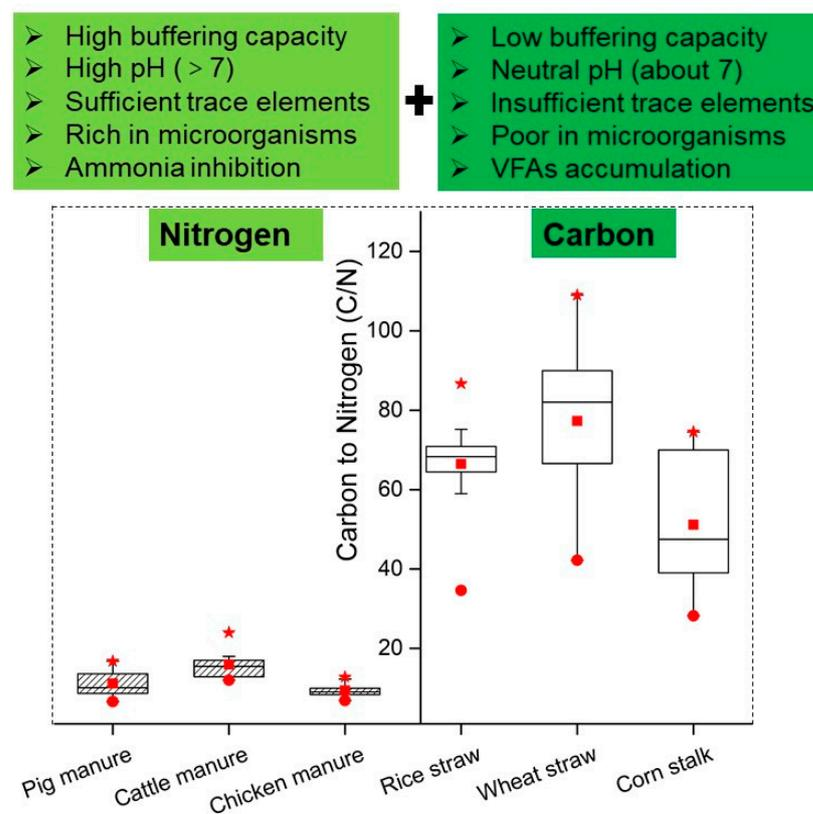
**Figure 2.** The principle of co-digestion using carbon-rich substrates (using crop straw as an example) and nitrogen-rich substrates (using livestock manure as an example). The carbon and nitrogen reflect total carbon and total nitrogen, respectively. For every substrate,  $n = 10$ . Note: Red stars indicate outliers.
