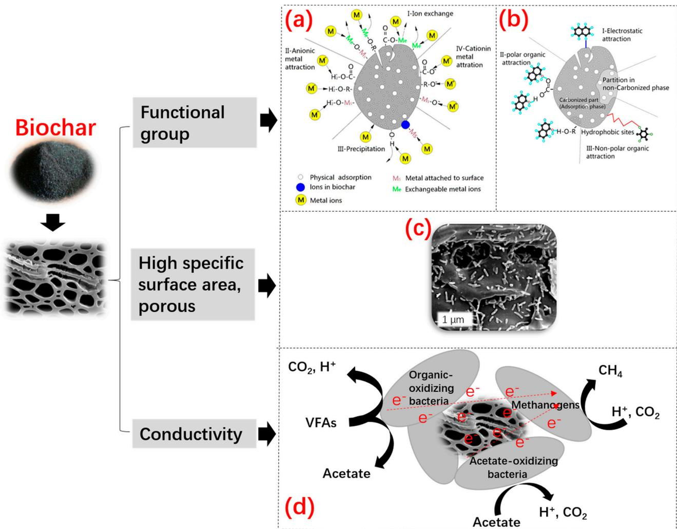
**Figure 9.** The mechanism of biochar in anaerobic digestion considering its three basic characteristics for (a,b) adsorption mechanism of inorganic pollutant and organic pollutant on biochar surface, (c) the function of biochar on immobilization of microorganisms, and (d) biochar-mediated direct interspecies electron transfer (DIET) (adapted from Ahmad et al. [160] and Baek et al. [161]).
