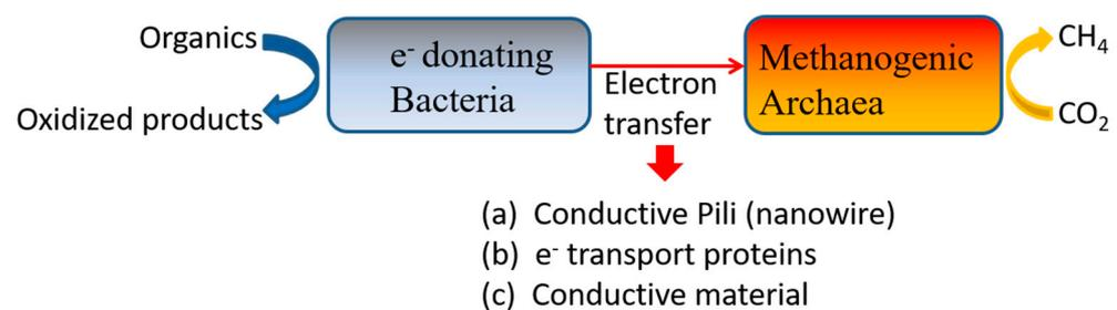
**Figure 6.** Three mechanisms of direct interspecies electron transfer (DIET) between organic-oxidizing bacteria and methanogenic archaea. This picture was adapted from Park et al. [9].
