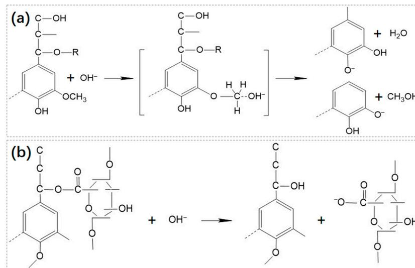
**Figure 1.** Schematic diagram of reaction mechanism between lignin, lignin complex, and  $\text{OH}^-$ . (a) The reaction mechanism between lignin and  $\text{OH}^-$ . (b) The reaction mechanism between lignin complex and  $\text{OH}^-$ . This picture was adapted from Yu et al. [48], with permission from Elsevier, copyright 2018.
