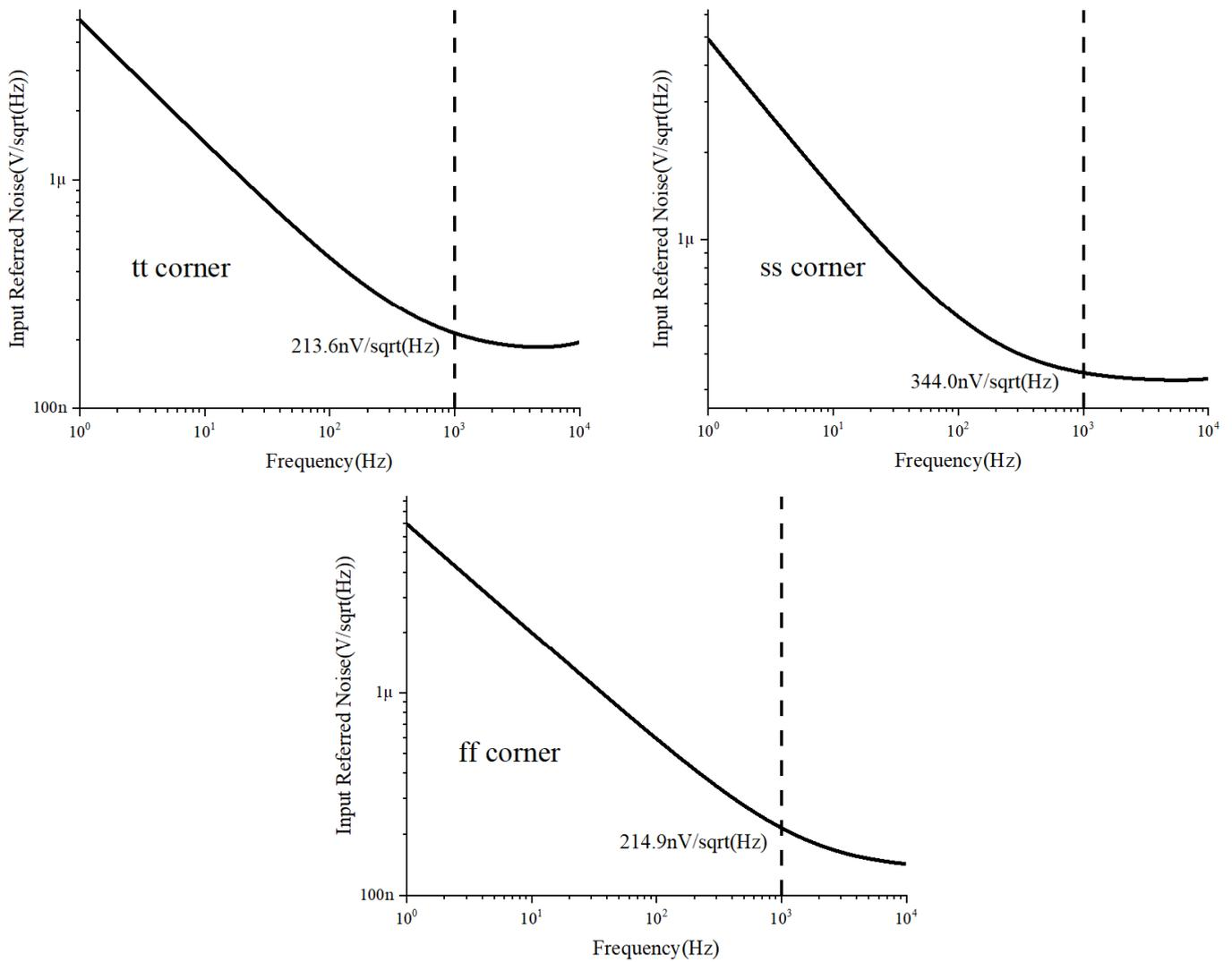
**Figure 20.** Input noise under 50 pF load.
