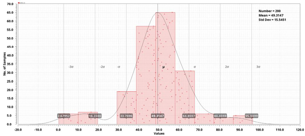
Figure 26. Histogram of CMRR under 200 runs of Monte Carlo simulations with estimated parasitics.
