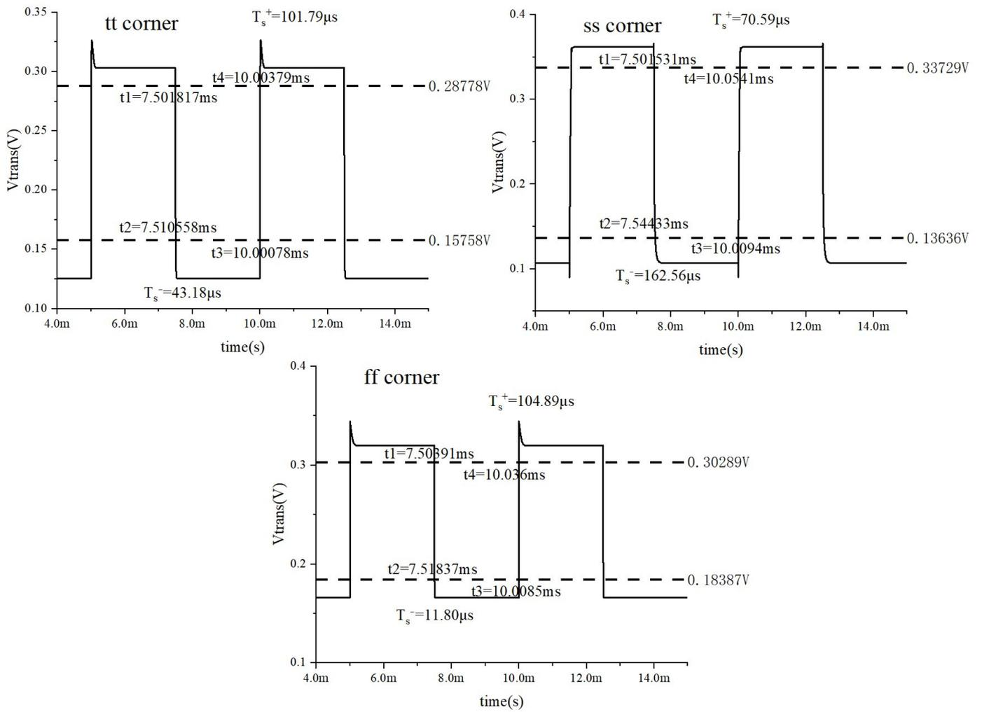
**Figure 19.** Transient response and slew rate of proposed amplifier.
