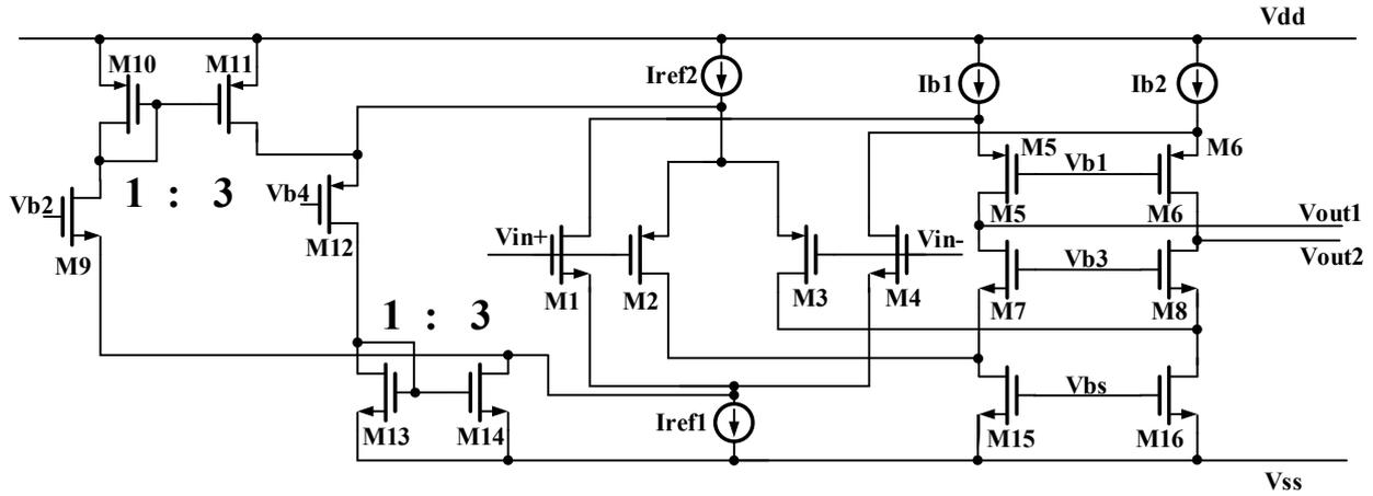
**Figure 9.** Gate-source driven rail-to-rail amplifier circuit with 3-to-1 ratio current mirror.
