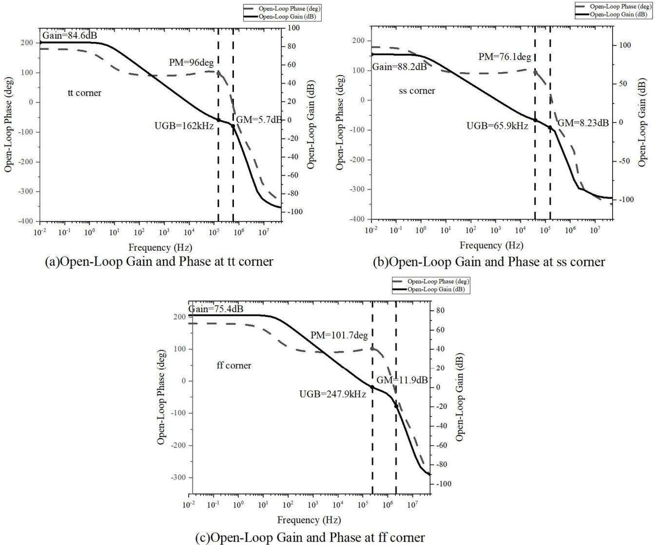
**Figure 13.** Open-loop gain under 50 pF load. (a) Open-loop gain and phase at tt corner. (b) Open-loop gain and phase at ss corner. (c) Open-loop gain and phase at ff corner.
