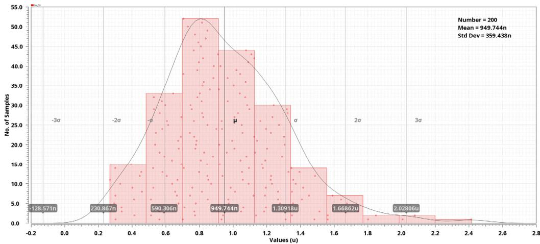
**Figure 29.** Histogram of  $P_w$  under 200 runs of Monte Carlo simulations with estimated parasitics.
