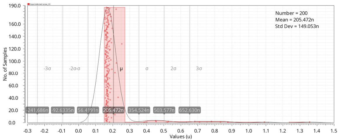
Figure 28. Histogram of noise under 200 runs of Monte Carlo simulations with estimated parasitics.
