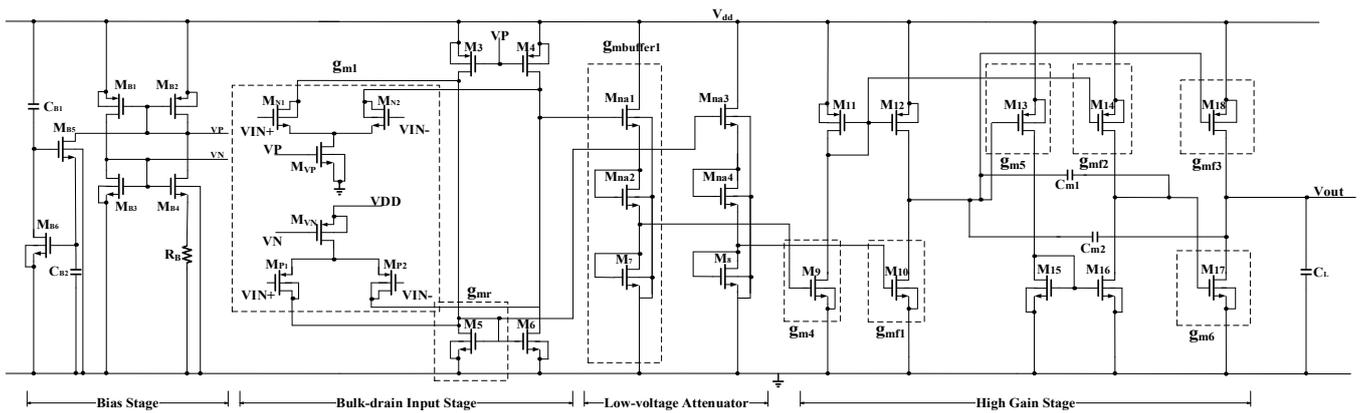
**Figure 10.** Circuit of the proposed amplifier.
