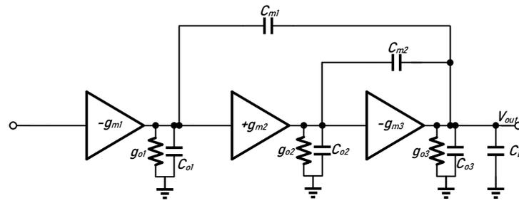
Figure 1. Topology of a three-stage NMC amplifier.
