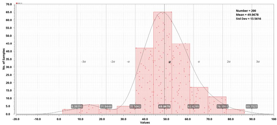
Figure 27. Histogram of PSRR under 200 runs of Monte Carlo simulations with estimated parasitics.
