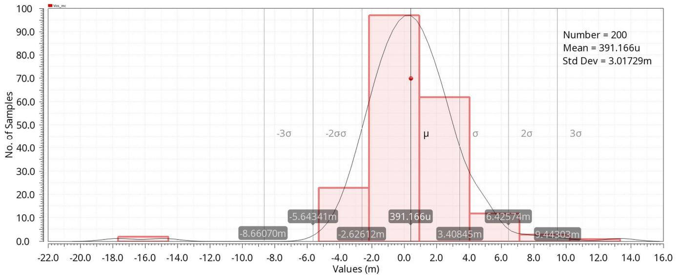
Figure 16. Histogram of offset voltage under 200 runs of Monte Carlo simulations at 50 pF load.
