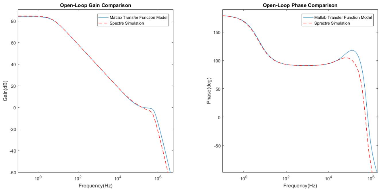
**Figure 30.** Comparison of open-loop results between spectra simulation and MATLAB models at 50pF capacitive load.
