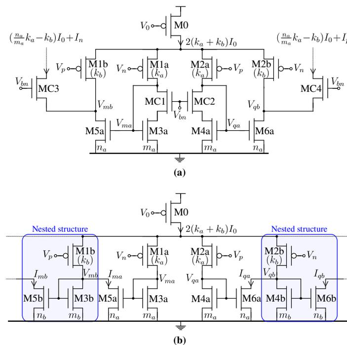
**Figure 12.** Schematic diagrams of: (a) transconductive core of the PMOS-input recycling folded cascode OTA, (b) transconductive core of the PMOS-input nested-mirror OTA.
