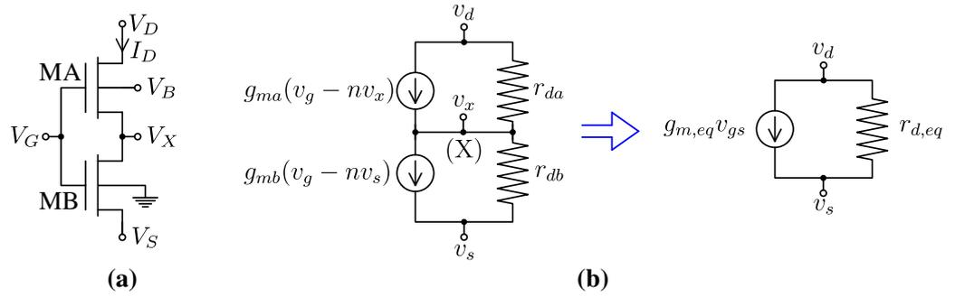
**Figure 15.** Schematic diagrams of the compound body-biased MOSFET (CBBM): (a) basic structure and (b) small-signal circuits.
