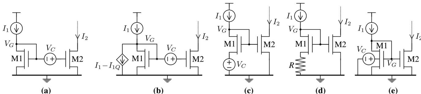
**Figure 13.** Schematic diagrams of non-linear current mirror configurations: (a) gate-series  $V_C(I_1)$ ; (b) same as previous but with constant  $V_G$ ; (c) source-series  $V_C(I_1)$ ; (d) trivial implementation of the previous by the means of a resistor; (e) body modulation at the input device.
