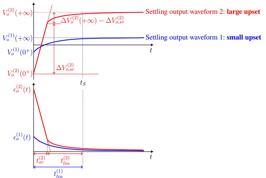
**Figure 2.** Chronograph of the differential output voltage  $V_o(t)$  [from (3)] the relative error  $\epsilon_o(t)$  [from (7)] for a small input step and for a large input.
