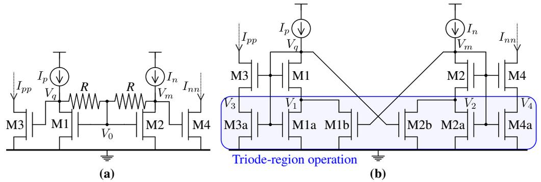
**Figure 14.** Schematic diagrams of differential non-linear current mirrors: (a) structure based on local common-mode feedback circuit (LCMF) and (b) structure based on the non-linear source degeneration.
