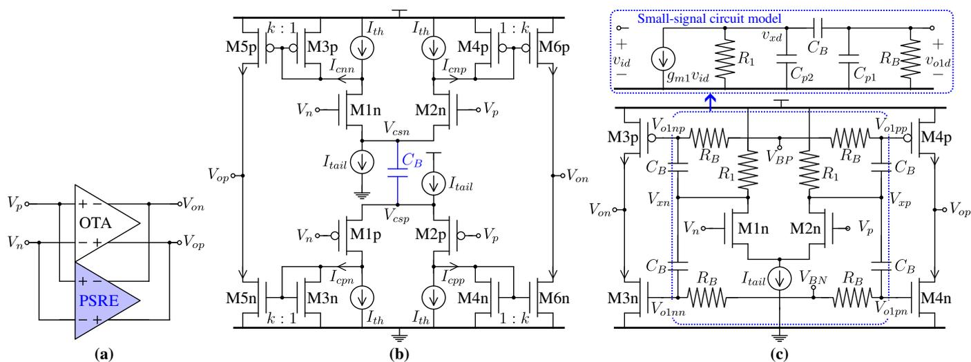
**Figure 16.** Schematic diagrams of (a) OTA+PSRE configuration; (b) Implementation of a PSRE based on current mirrors, enhanced by the boost capacitor  $C_B$ ; (c) Implementation of a class-B PSRE based on RC-bias ties.
