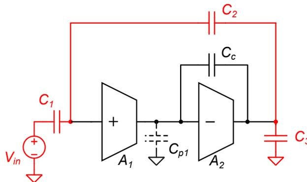
**Figure 6.** Simplified single-ended equivalent circuit of a two-stage amplifier with capacitive feedback.
