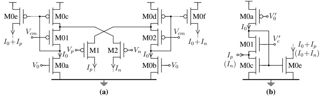
**Figure 11.** Schematic diagrams of Flipped Voltage Follower employed as (a) current buffer loop for class-AB current biasing, (b) low-voltage current mirror.
