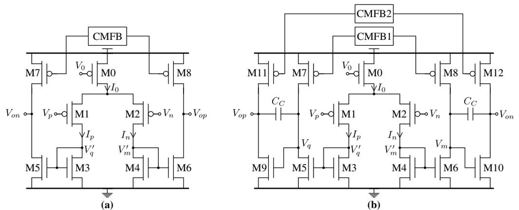
**Figure 5.** Schematic diagrams of (a), a PMOS-input mirror OTA; (b), a two-stage Miller-compensated PMOS-input OTA.
