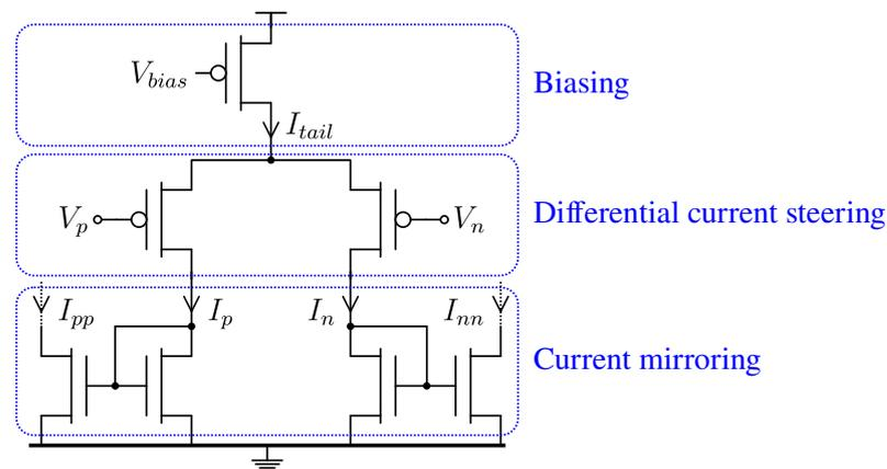
**Figure 10.** Schematic diagram of the functional parts of a mirror-based OTA.
