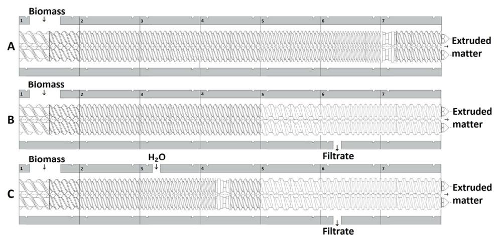
**Figure 2.** Schematic representation of the three screw profiles tested in the Clextal BC 45 twin-screw machine. (A) Soft extrusion, (B) high-shear extrusion and (C) high-shear extrusion with rehydration.
