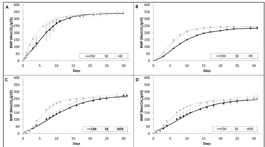
**Figure 4.** Experimental BMP (square symbols) and BMP kinetics using the modified Gompertz equation model (lines) before and after twin-screw extrusion pretreatment: (A) SB, (B) WT, (C) CS and (D) WS. BMPs from HE/HER samples were assessed after mixing extrudate and filtrate samples in the same proportions as at the extrusion outlet.
